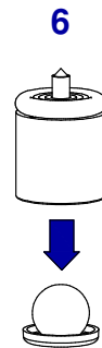
6 PLACE METERING PIN INTO THE CAP. PLACE BALL INTO THE SEAT, AS SHOWN. PRESS CAP DOWNWARD ONTO THE BALL/SEAT COMBINATION UNTIL THE CAP BOTTOMS OUT ONTO A TABLE OR SMOOTH CLEAN SURFACE
