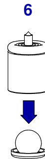
6 PLACE METERING PIN INTO THE CAP. PLACE BALL INTO THE SEAT, AS SHOWN. PRESS CAP DOWNWARD ONTO THE BALL/SEAT COMBINATION UNTIL THE CAP BOTTOMS OUT ONTO A TABLE OR SMOOTH CLEAN SURFACE
