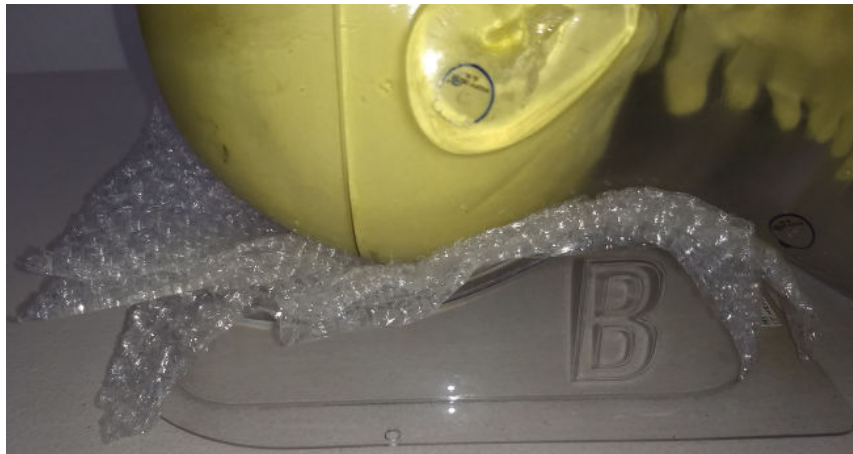
Figure 6.1.1. Phantom showing the use of a Silverman headrest with bubble wrap.
