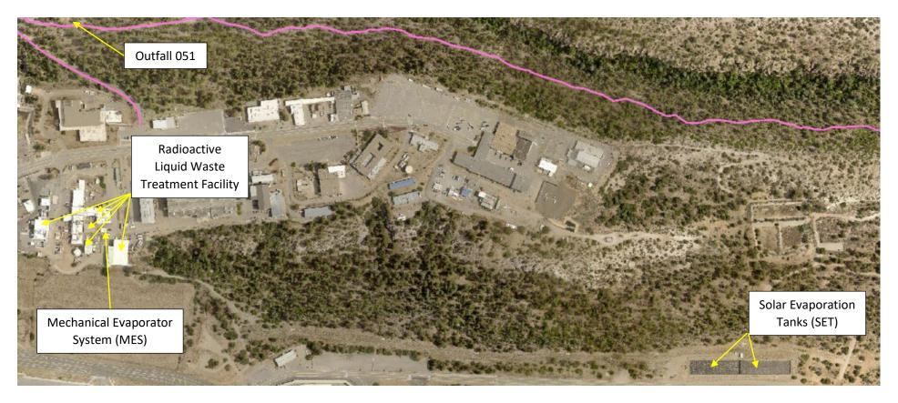
Photograph - NPDES-051-19-001 Location of the Radioactive Liquid Waste Treatment Facility, Mechanical Evaporator System (MES), Solar Evaporation Tanks (SET), and Outfall 051
