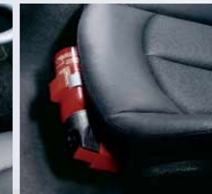
Mounting for fire extinguisher
