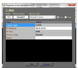
3 Select **Densité Frame** as the Device Type and enter device properties as below:
