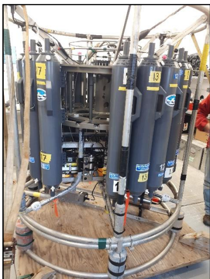
Figure 6. CTD electronics and D2 logger inside the ring of Niskin bottles.
