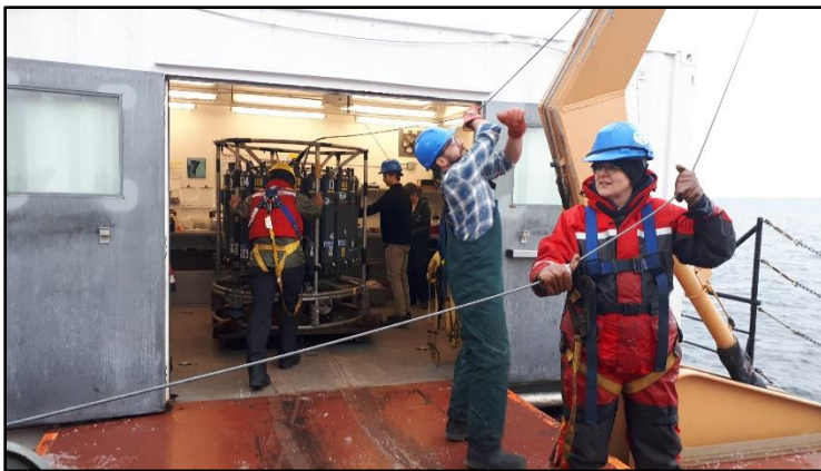
Figure 5. Recovered rosette being brought in for sampling.
