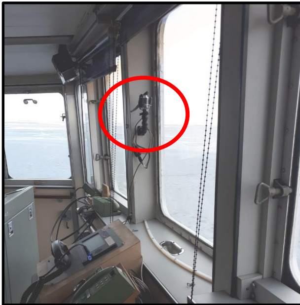
Figure 13. The downward and forward looking netcams above the bridge.
