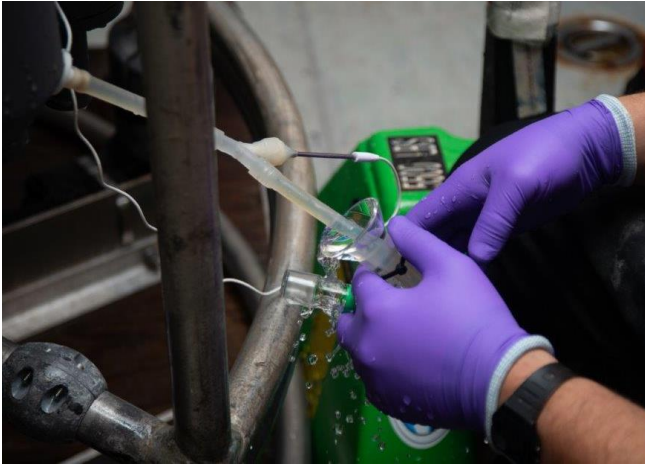
Figure 9. Oxygen sampling from the rosette. Photo by Fred Marin (2019).
