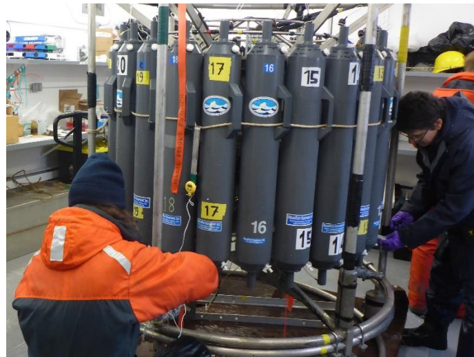
Water sampling around 24 bottle rosette
