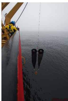
Figure 12. Bongo nets being deployed from the foredeck, photo Gary Morgan, JOIS 2021
