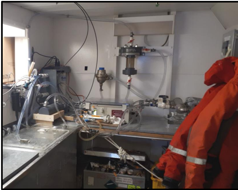
Figure 15. Seawater loop system w/ Chl-a and FDOM sensors attached to left wall, the second FDOM sensor in wood cradle and pCO 2 system on bench in center. The seawater loop provides uncontaminated seawater from 9m depth to the science lab for underway measurements
