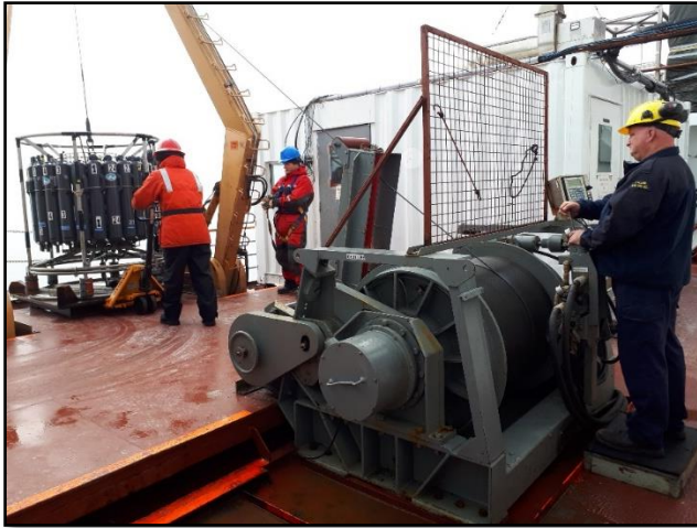
Figure 3. Rosette operation on deck with Hawboldt winch and Brooks Ocean Instrumented Sheave display box mounted on the right.
