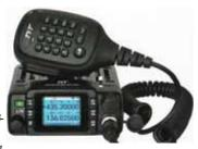
Temperature -30C+60C Operating Voltage 13.8V DC Dimension 107\*125\*45mm
