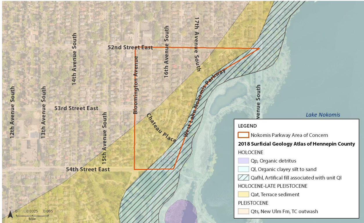
Figure 15: 2018 Surficial Geology for the Nokomis Parkway Area of Concern. Excerpt from the 2018 Surficial Geology Atlas of Hennepin County for the Nokomis Parkway Area of Concern shows homes were built over areas of Lake Nokomis that were drained and filled. (Credit: MCWD; Data Source: Steenberg et al., 2018)
