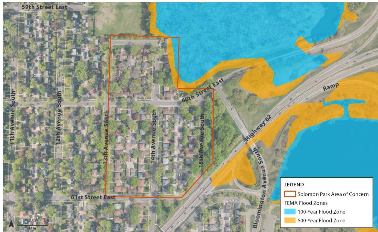
Figure 25. FEMA Flood Zone for the Solomon Park Area of Concern. FEMA flood insurance rate map (FIRM) for the Solomon Park Area of Concern which shows some properties are located with the 100-year floodplain. (Credit: MCWD)
