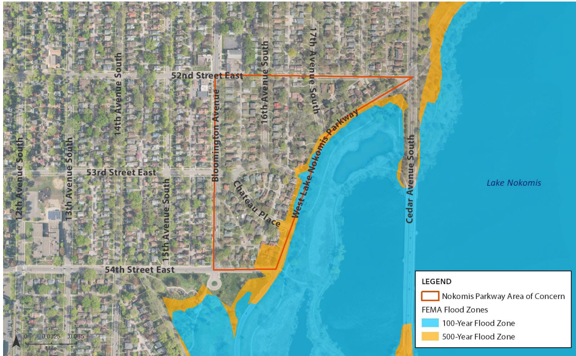
Figure 17: FEMA Flood Zone for the Nokomis Parkway Area of Concern. FEMA flood insurance rate map (FIRM) for the Nokomis Parkway Area of Concern. (Credit: MCWD)
