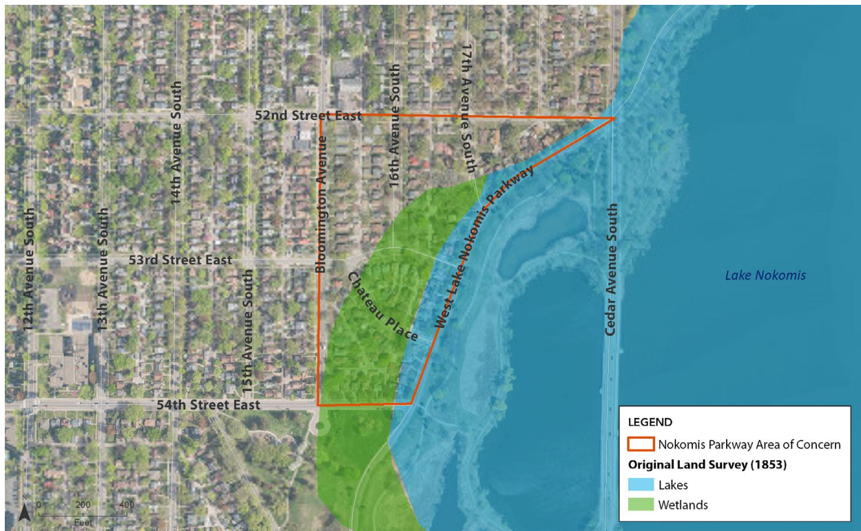
Figure 43: 1853 Land Survey for the Nokomis Parkway Area of Concern. The Nokomis Parkway Area of Concern boundary is overlaid on the 1853 land survey, which shows homes were built over a former wetland and the former basin of Lake Nokomis. (Credit: MCWD; Data Source: GLO Historic Plat Maps)
