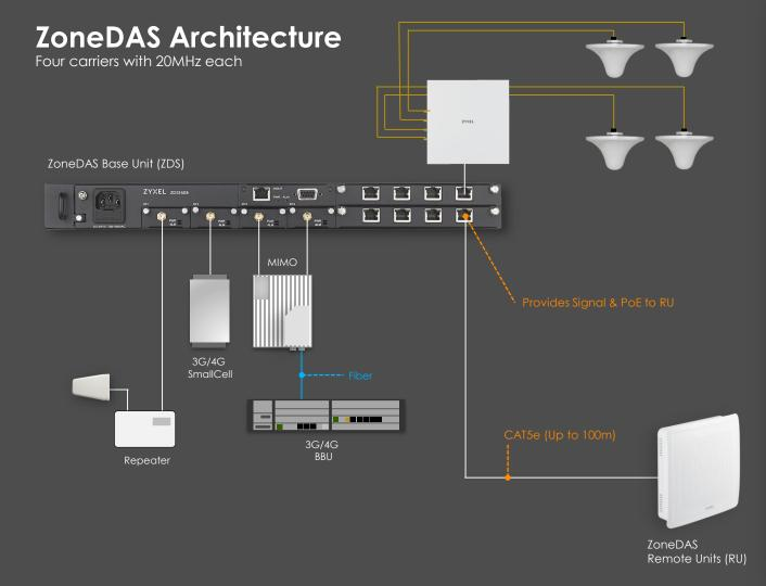
ZYXEL Tu **RU Output power** configurable from 14~23 dBm
