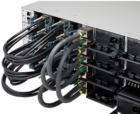
Figure 9. StackWise-480 and StackPower connectors
