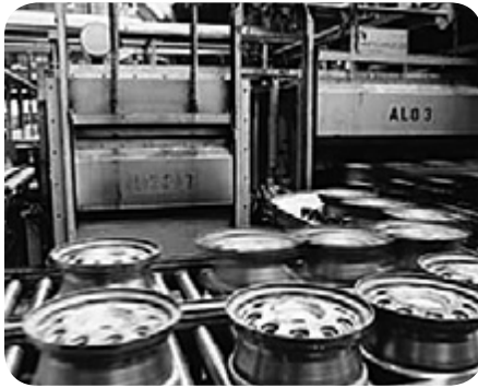
Aluminium industry: curing oven for wheel rims
