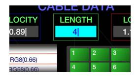
Press the "CALC" button to recalculate the Velocity Factor based on the newly entered cable length. There is no need to run a new capture. In thie way you can calculate the velocity factor for a new cable with a known length.
