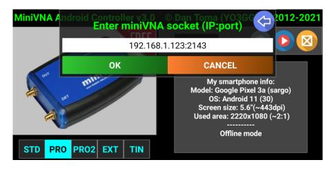
Enter the data in the format *IPaddr:port* (or *hostname:port*) and then press OK. Connection will be established automatically, Status panel will go green and the Wi-Fi symbol will be displayed on top of the miniVNA image.
