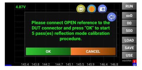
A progress message will be displayed. When the OPEN calibration is completed, remove the OPEN calibration reference from the DUT connector. For the miniVNA Pro, connect the SHORT (0 ohm) calibration reference to the DUT connector as shown in the following picture and press the "OK" button again.
