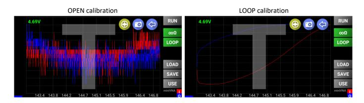
**NOTE:** For both Reflection and Transmission Calibration, the vertical scale of the graph is in relative units, with no other meaning. The graph uses auto scale to better represent the trend which must be similar for miniVNAs of the same model.
