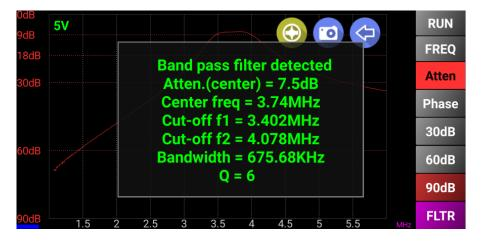
The application can automatically detect (in most situations) the filter type (low pass, band pass, band reject or high pass), adjusting the calculated parameters accordingly. Please be aware that this is still an experimental feature, so it may fail with some filters. Click on the data box to remove it from the screen.
