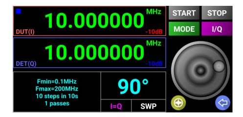
To set the SWEEPER (SWP) parameters long press on "MODE" button when in SWP mode or press the area containing sweeper configuration data in the lower left part of the screen. An overlay will be displayed which will help you to set the parameters values as follows:
