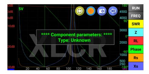
After the capture you can activate the first marker (yellow) to display some other parameters for a specific frequency. Where the Xs value is negative, an equivalent capacity is calculated based om formulas from <u>here</u>. Where XS is positive, an equivalent inductance is calculated.
