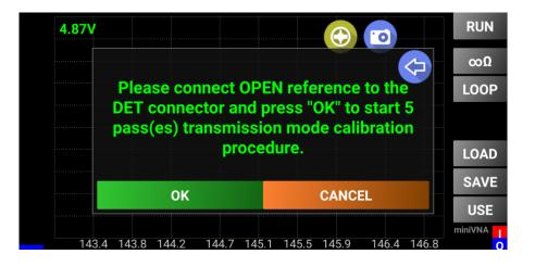
When completed, remove the OPEN reference from the DUT connector.
