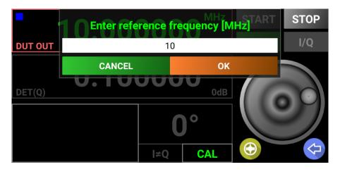
Enter the reference frequency in MHz and press "OK". Reference frequency will be displayed. Start LIVE mode and change the frequency with the tuning knob till the generator output exactly the reference frequency, then press SAVE.
