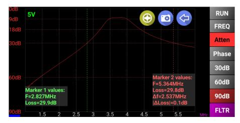
Long press on the "Atten" button to automatically measure the bandwidth at a specific attenuation.
