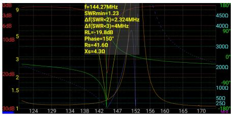
Besides the values for the selected parameter values, the bandwidth ( $\Delta f$ ) for a SWR < 3:1 and for a SWR < 2:1 will be displayed too. If minSWR is > 3:1, then the bandwidth value will not be displayed.
