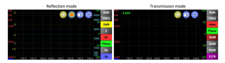
On the left side are the scales for SWR and Loss. On the right side are the scales for Z, Rs, Xs (all in ohms) and Phase (in degrees). Phase is between -180 and 180 for the miniVNA Pro and between 0 and 180 for the miniVNA standard. Xs has an absolute value for the miniVNA standard and a signed value for miniVNA Pro. Negative value for Xs is displayed as a dashed line on the graph.
