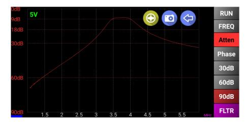
Pressing the "FLTR" button some of the filter parameters will be automatically calculated.
