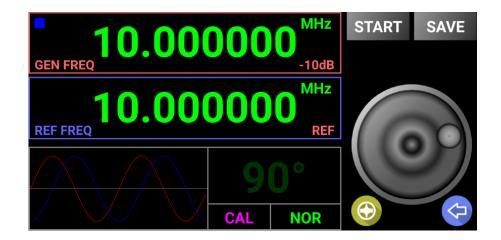
To calibrate, use a very well calibrated frequency meter connected to DUT (miniVNA Pro without extender or miniVNA standard) or TX (miniVNA Pro with Extender). The available frequency range is the one supported by your miniVNA model (0.1-180 MHz for miniVNA Standard, 0.1-200 MHz for Pro without Extender and 40-1500 MHz for Pro with Extender). In this example, the miniVNA will be calibrated using a 10 MHz reference.
