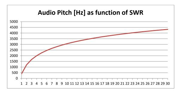
When using this function, adjust for the lowest pitch and when this has been found, look at the display in order to see the actual SWR value.
