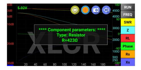
4. Unknown component (a 1m piece of RG316 cable):
