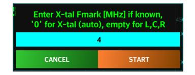
To manually measure X-tal parameters, enter the frequency marked on the X-tal case and press START. A data capture around the marked frequency will start. At the end, you will get the exact resonance frequency and the quality factor.
