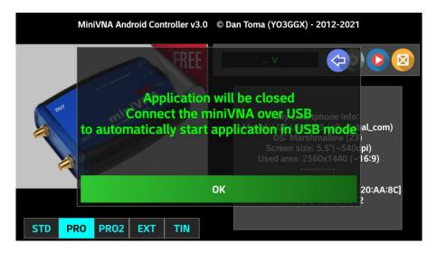
Connect your miniVNA over USB through an UTG adapter and provided USB cable, or an USB-C(male)/USB-B(male) cable (miniVNA Standard, Pro or Pro2) or USB-C(male)/miniUSB(male) cable (for Tiny) if your Android devices use USB-C type connector.
