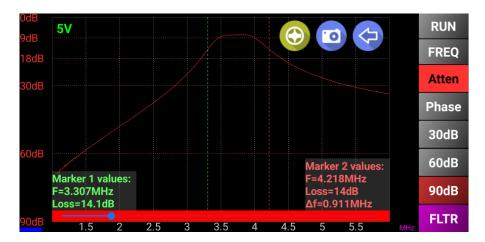
Two markers will be displayed and a red slider in the bottom of the screen. Move the slider left or right do decrease/increase the attenuation to be considered for the bandwidth measurement.
