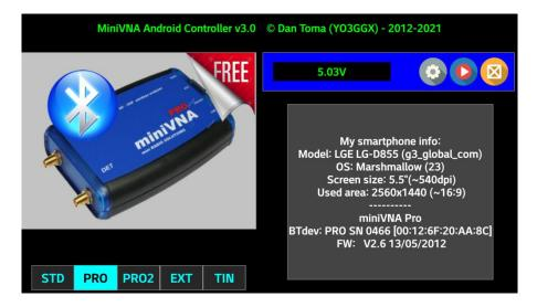
**NOTE:** The battery voltage text color will change to yellow when low level and to red when critical. When red, recharging the miniVNA battery is mandatory to prevent battery damage. If your analyzer use an external power, the displayed voltage can be even over 5V.
