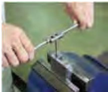
Manual tapping by using tap wrench
