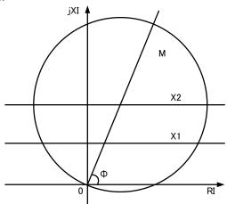
Figure 1 Conceptual diagram of distance relay
