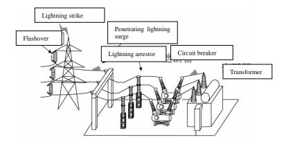
Figure 1 Conceptual diagram of lightning surge calculation in air insulated substation
