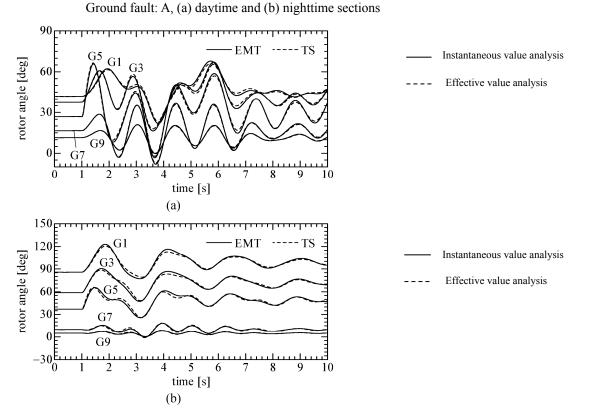
Figure 4 Comparison of the results of instantaneous value analysis using XTAP and effective value analysis using CPAT
