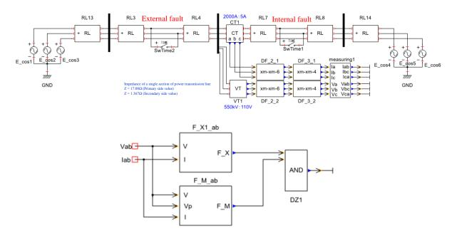
Figure 7 Analysis circuit and relay sequence
