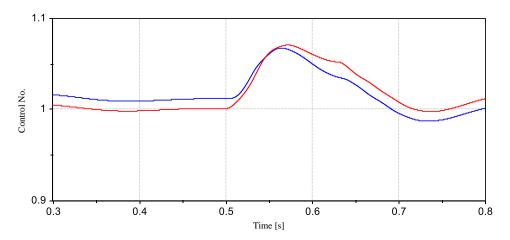
Figure 2 DC capacitor voltage (average value of all cells) [pu] (the reference voltage is 125 kV).
