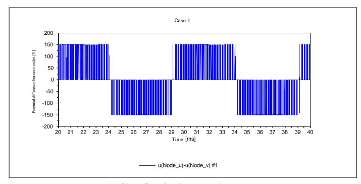
(a) Line-to-line voltage between u and v
