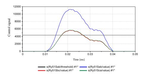
Figure 11 51S calculation value at one cycle interruption (the black line is the settling value)
