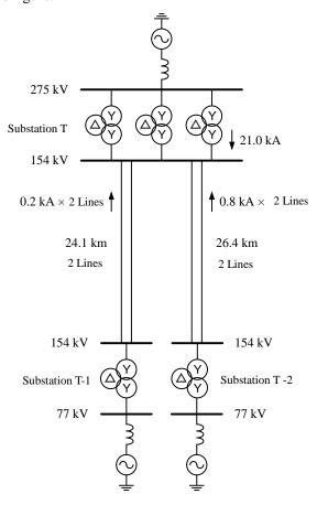
Figure 1 Single-line diagram of model system
