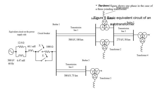
Figure 4 Example circuit for the calculation of input surge owing to block energization
