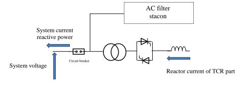
Figure 3 Voltage and current measurement points
