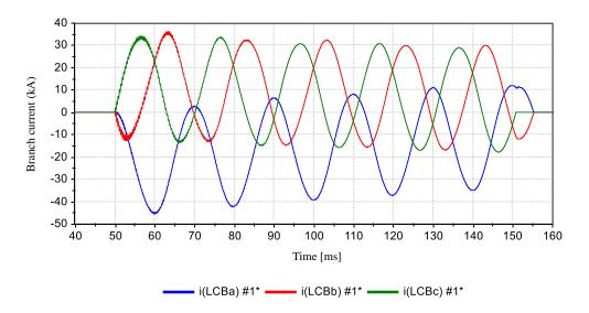
Figure 6 Current waveform of circuit breaker
