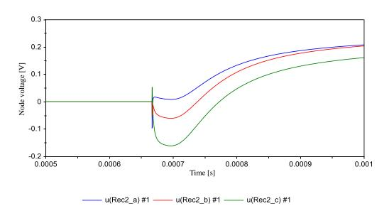
(b) Far-end voltage waveform of the second circuit
