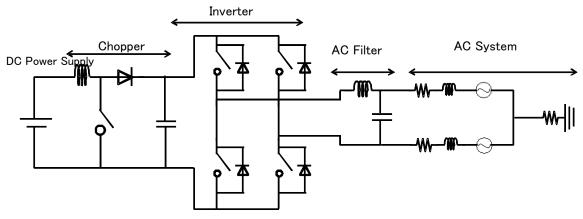
Figure 1 Analysis circuit
