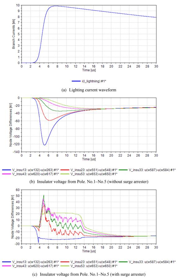
Figure 8 Calculation results obtained by the Heidler function lighting current waveform
