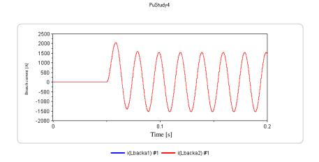
The graph was plotted by superimposing the current of phase A on the 66-kV side. This indicates that the conversion was carried out satisfactorily. The method of conversion is as follows.
