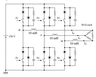
Figure 1 Analysis circuit
