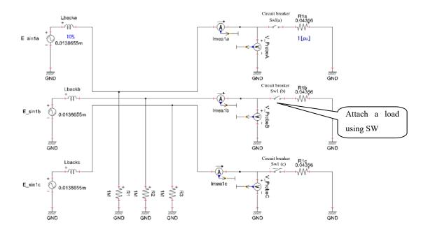
Figure 1 Analysis circuit
