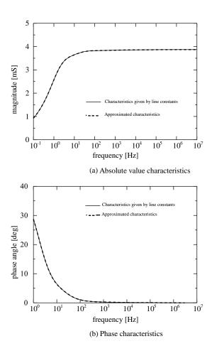
Figure 4 Results of frequency characteristic approximation of the characteristic admittance matrix component (1, 1)
