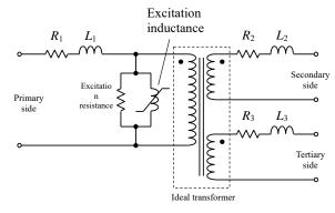
$R_1$ ,  $L_1$ : Resistance and leakage inductance of the primary winding  $R_2$ ,  $L_2$ : Resistance and leakage inductance of the secondary winding  $R_3$ ,  $L_3$ : Resistance and leakage inductance of the tertiary winding
