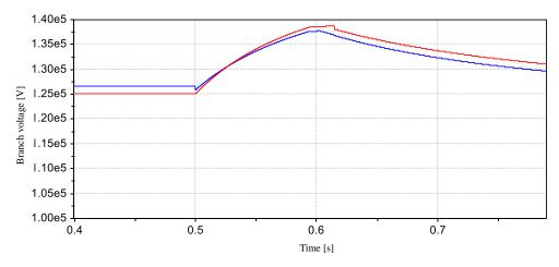
Figure 2 DC voltage [pu]: blue line:, terminal 1; red line, terminal 2 (reference voltage of 125 kV)
