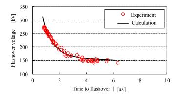
Figure 4 Example of *V-t* characteristics of a distribution insulator.
