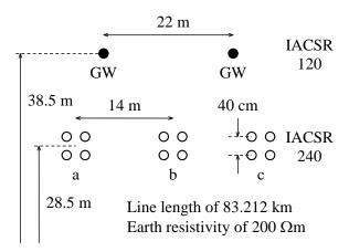
Figure 1 Assembly of 500-kV horizontally arranged single line transmission line
