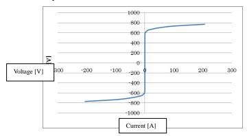
Figure 4 Example of V-I characteristics of varistor between the lines of electronic WHM
