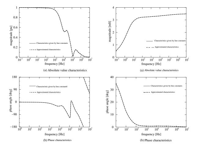
Figure 3 Approximation of frequency characteristics of the propagation function matrix component (1, 1)
