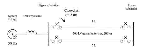
Figure 1 Skeleton diagram of a grid in which an input surge calculation is conducted
