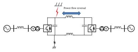
Figure 1 Analysis circuit
