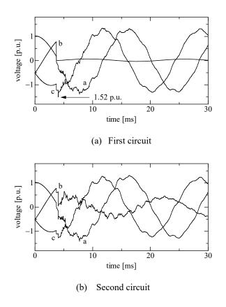
Figure 6 Calculation results at the time of occurrence of ground-fault when the phase of the source voltage is  $50^{\circ}$
