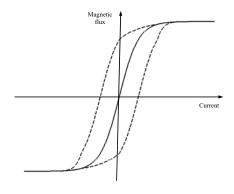
Figure 2 Hysteresis characteristics of iron core
