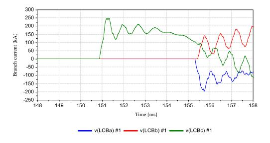
Figure 7 TRV waveform at the time of BTF interruption
