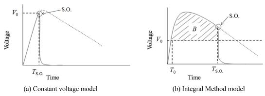
Figure 3 Overview of insulator flashover model
