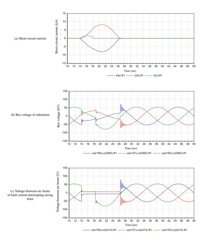
Figure 6 XTAP execution result (current interruption time of fault current interrupting arcing horn: 1 half wave)
