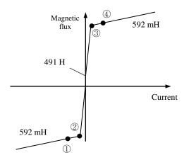
In XTAP, when specifying the nonlinear characteristics of the parts based on polygonal lines, the characteristics outside the specified range are calculated through a linear extrapolation.
