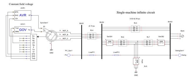
Figure 2 Model system created in XTAP
