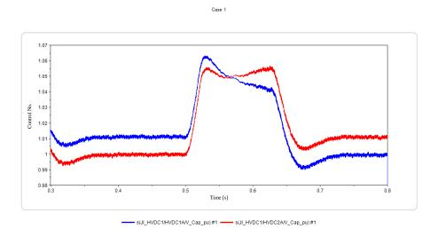
Figure 3 DC voltage [pu] Blue line, terminal 1; red line, terminal 2 (the reference voltage is 125 kV)
