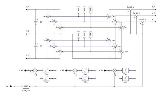
Fig. 3 Average value model for the three-level NPC bridge.
