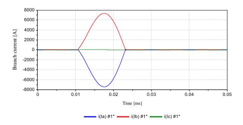
Figure 3 Current waveform at 0.5 cycle interruption
