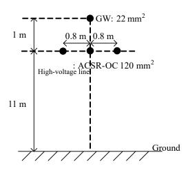
Figure 3 Pillar assembly of high-voltage cable and overhead ground wire
