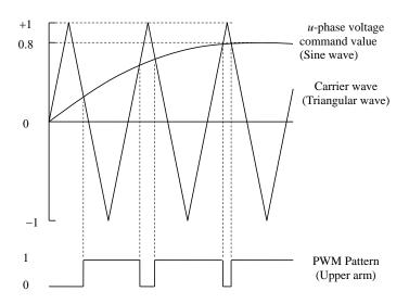
Figure 2 Triangular wave comparison method
