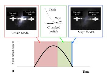
Figure 3 Current breaking simulation model of fault current interrupting arcing horn
