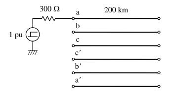
Figure 2 Surge propagation simulation circuit
