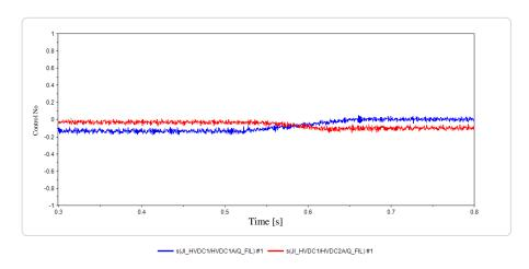
Figure 6 Reactive power [pu] Blue line, terminal 1; red line, terminal 2 (the reference capacitance is 55.9 MVA)
