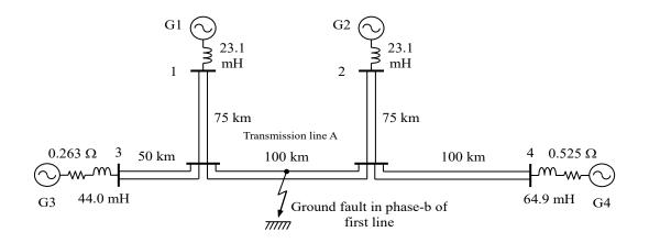
Figure 3 Example circuit of ground-fault surge calculation
