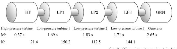
(shaft stiffness in pu torque/electrical rad)
