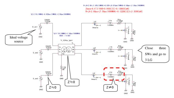
Figure 1 Analysis circuit
