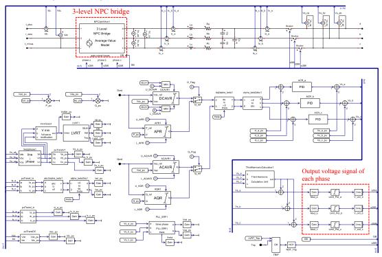
Fig. 2 Internal configuration of the three-phase PCS (average value model)
