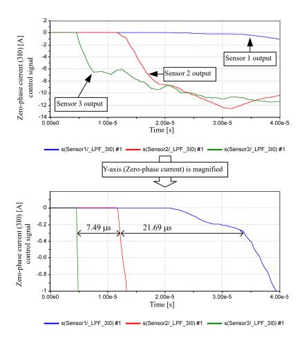
Figure 7 Output of each sensor and surge arrival time difference when ground-fault occurs at "ground-fault point Case 1"
