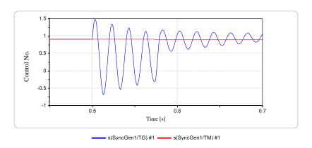
(i) Mechanical and magnetic torque [pu] Figure 4 Analysis results using XTAP
