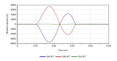
Figure 9 Current waveform at one cycle interruption
