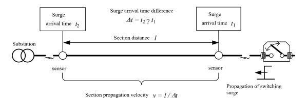
Figure 2 Acquisition of surge propagation speed
