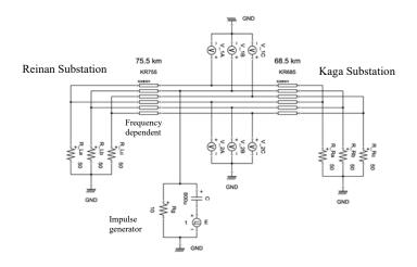
Figure 8 XTAP data reproducing the ground-fault surge test of Kaga-Reinan line
