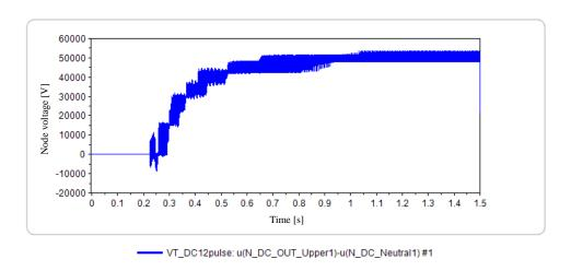
Figure 5 DC voltage waveform at startup (DC voltage ①)
