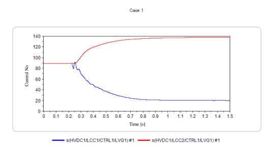
Figure 8 Control angle α Red line, 50-Hz side; blue line, 60-Hz side
