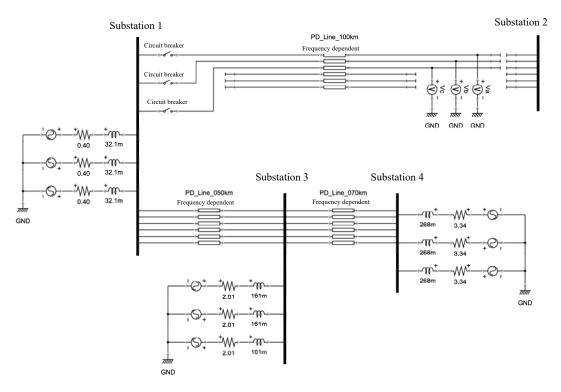
Figure 11 XTAP data for switching surge calculation
