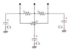
Figure 4 Pole-mounted transformer model
