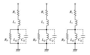
Figure 8 Equivalent circuit of a load
