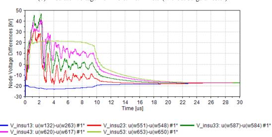
(c) Insulator voltage from Pole. No.1–No.5 (with surge arrester)
