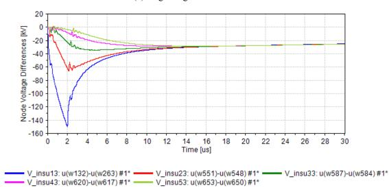
(b) Insulator voltage from Pole. No.1–No.5 (without surge arrester)
