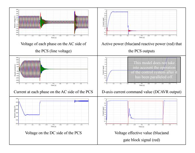
Fig.3. PCS response when an instantaneous voltage drop assuming an 3LS fault in the high voltage distribution line.
