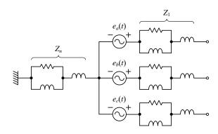
Figure 7 Equivalent circuit of the power supply side considering its frequency dependence
