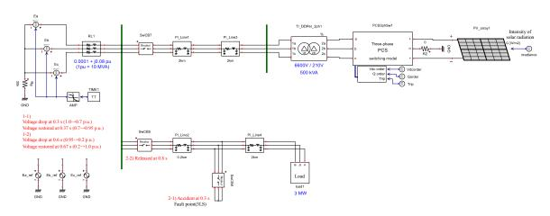
Fig. 1 Circuit diagram of the high-voltage distribution system simulated on the XTAP and the utility-scale solar system connected to it.
