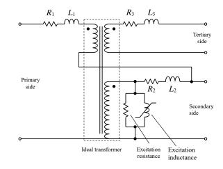
$R_1$ ,  $L_1$ : Resistance and leakage inductance of the primary winding  $R_2$ ,  $L_2$ : Resistance and leakage inductance of the secondary winding  $R_3$ ,  $L_3$ : Resistance and leakage inductance of the tertiary winding
