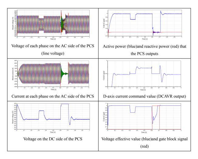
Fig.2. PCS response when an instantaneous voltage drop occurs, assuming 3LG-O in the upper system
