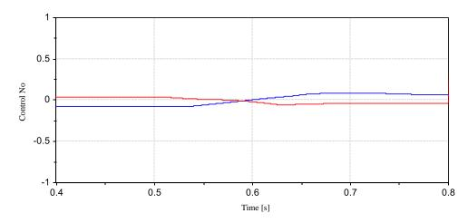
Figure 5 Reactive power [pu]: blue line, terminal 1; Red line, terminal 2 (the reference capacity is 55.9).
