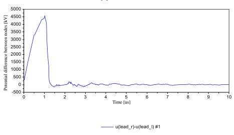
(c) Waveform of voltage between horns
