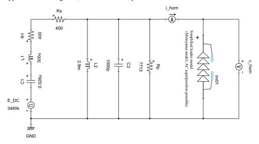
Figure 1 Analysis circuit
