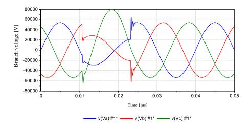
Figure 4 Voltage waveform at 0.5 cycle interruption
