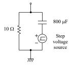
(b) Equivalent circuit of impulse generator
