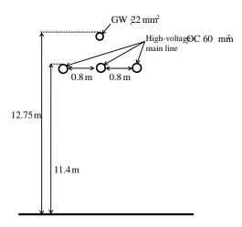
Figure 2 Conductor arrangement in high-voltage distribution line
