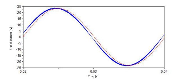
Blue line, AC current before passing through the filter; red line, AC current after passing through the filter
