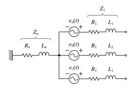
Fig. 6 Equivalent circuit of the power supply side
