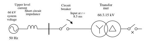
Figure 1 Single line connection diagram of analysis circuit
