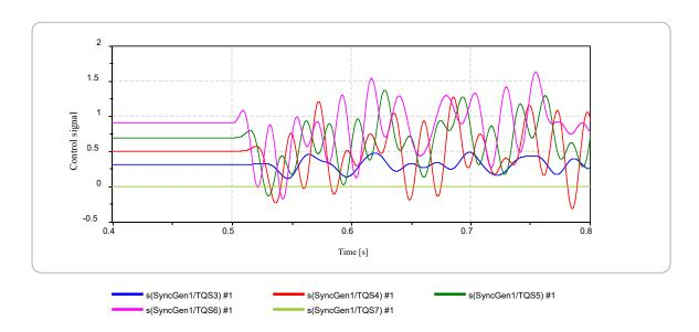
Figure 5 Torsional torque of each mass point (between adjacent mass points on the right-hand side in Figure 1)
