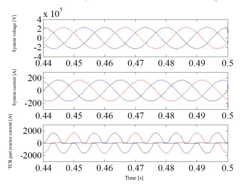
Figure 4 Voltage and current waveforms during a steady state
