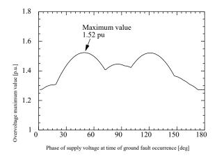
Figure 5 Maximum voltage versus phase of source voltage at time of occurrence of ground-fault
