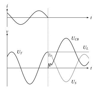
Figure 4 Illustration of TRV waveform of capacitive
