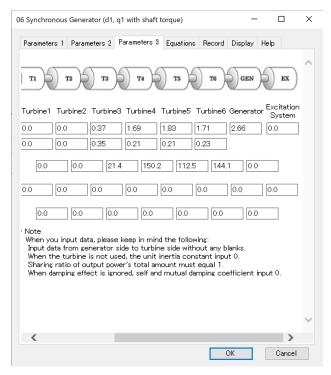
Figure 2 Shaft data input screen of synchronous generator
