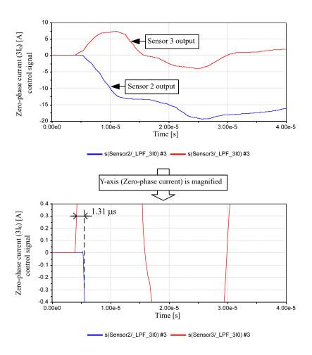
Figure 9 Outputs of sensors 2 and 3 and the difference in surge arrival time when a ground-fault occurs at "Ground-fault point Case 3"
