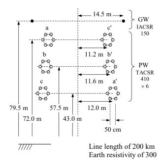
Figure 2 Assembly of 500-kV vertically arranged double-circuit transmission line
