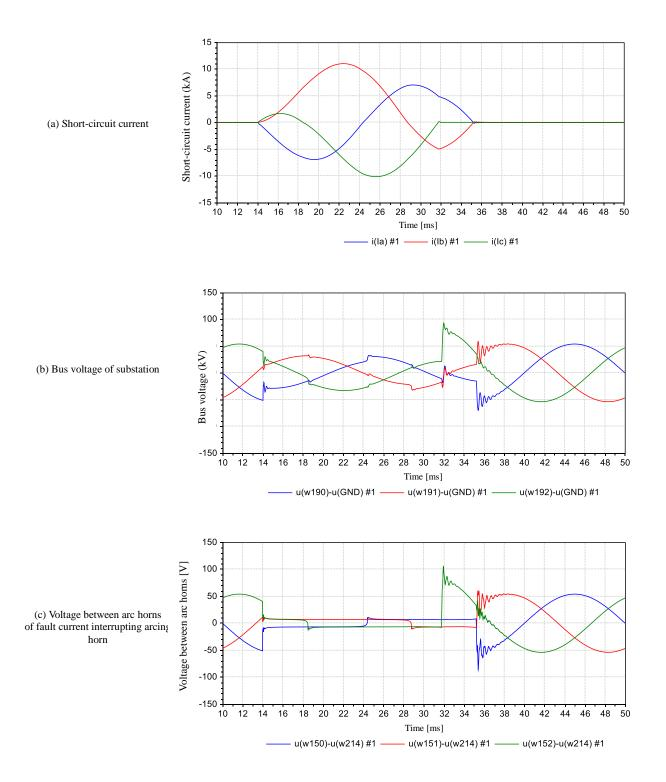
Figure 5 XTAP execution result (current interruption time of fault current interrupting arcing horn: 2 half waves)
