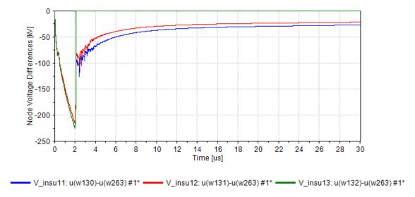
(a) Case without surge arrester (Peak value of lightning current: 15 kA, Flashover at Pole No. 1)
