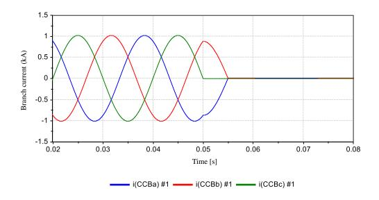
Figure 8 Current waveform at the time of capacitive current switching
