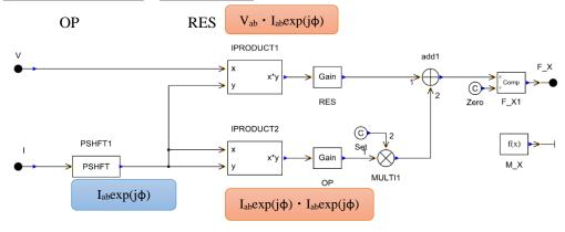
Figure 6 Modeling of reactance elements
