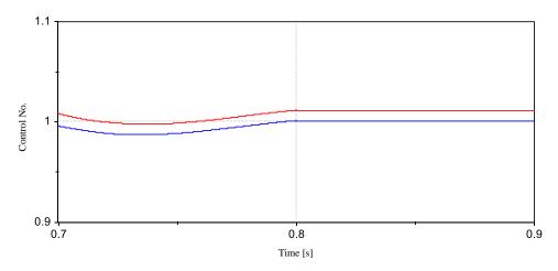
Figure 6. DC voltage [pu]: blue line, terminal 1; red line, terminal 2 (the reference voltage is 125 kV, and is the average value of the capacitor voltages of 6 arms)
