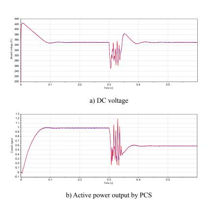
Fig. 6 Comparison 3 of the switching model and average value model (Blue: switching model, Red: average value model)
