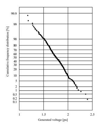
Figure 1 Cumulative frequency distribution of voltages generated by switching surge
