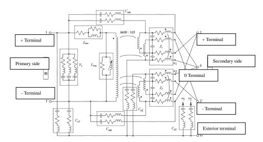
Figure 3 Example of the analytical model of pole-mounted transformer
