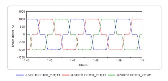
Figure 6 Transformer primary side current
