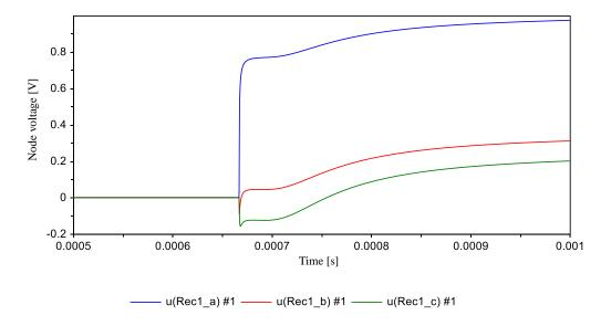
(a) Far-end voltage waveform of the first circuit
