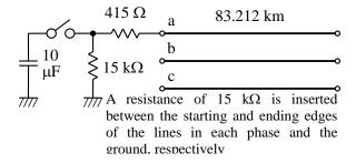
Figure 2 Surge propagation characteristic test circuit
