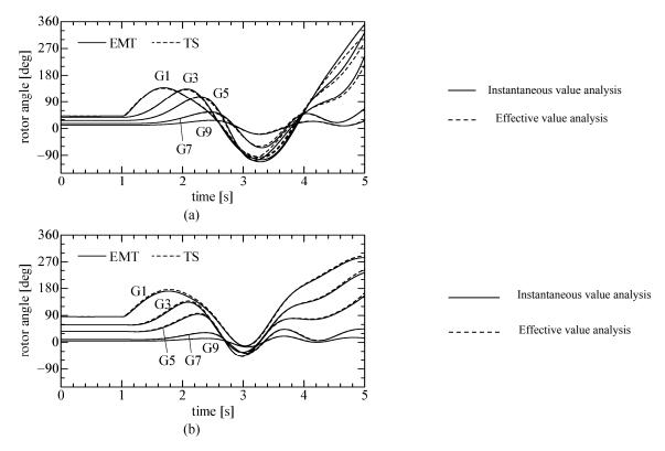
Figure 3 Comparison of the results of instantaneous value analysis using XTAP and effective value analysis using CPAT
