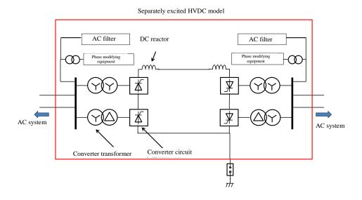
Figure 2 Schematic diagram of model
