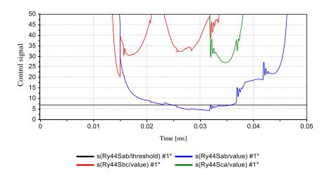
Figure 13 Calculated value of 44S at one cycle interruption (the black line is the settling value)
