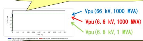
It can be seen that even in the pu system, the difference in the A phase voltage occurs when an active power flows in the transmission line of the inductance owing to the relationship
