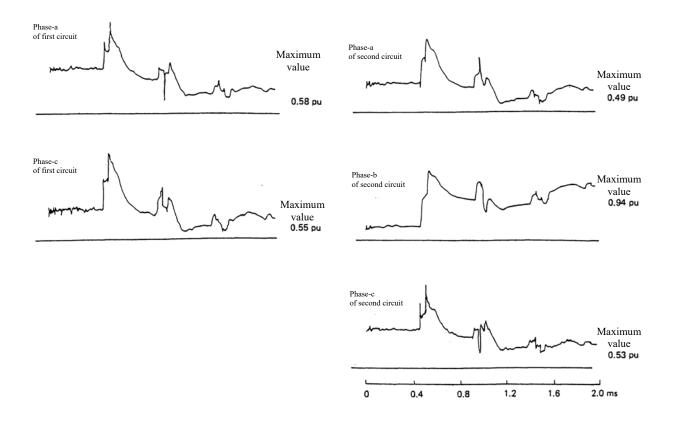
Figure 9 Measured results of ground-fault surge test at Kaga-Reinan line
