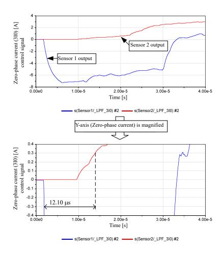
Figure 8 Output of sensors 1 and 2 and difference in surge arrival time when the ground-fault occurs in "ground-fault point Case 2"
