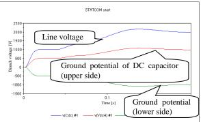
Converter transformer ab line voltage [V] on secondary side Line voltage of DC circuit and ground potential [V]
