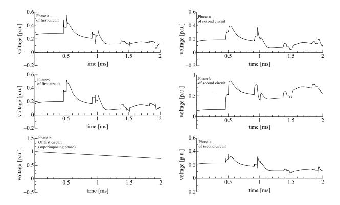
Figure 10 Calculation results of Kaga-Reinan line ground-fault surge test using XTAP
