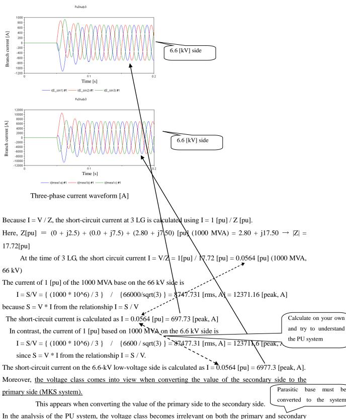
In the analysis of the PU system, the voltage class becomes irrelevant on both the primary and secondary sides, and the effective and instantaneous value analyses are the same. Consequently, the relaxed responses of the fundamental waves in the results of the effective and instantaneous value analyses
