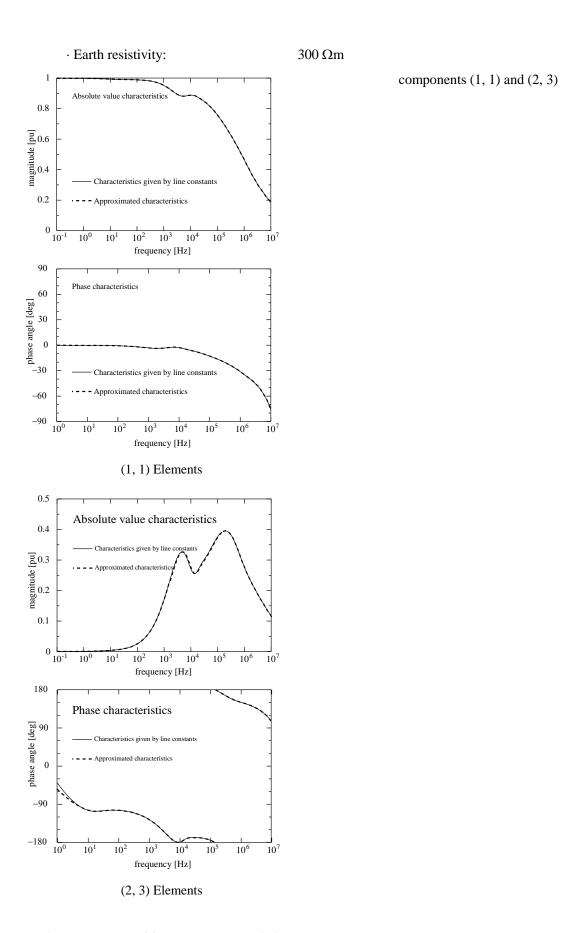
Figure 3 Results of frequency characteristic approximation of the propagation function matrix
