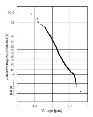
Figure 12 Cumulative frequency distribution of the voltages generated at the end of transmission line 1
