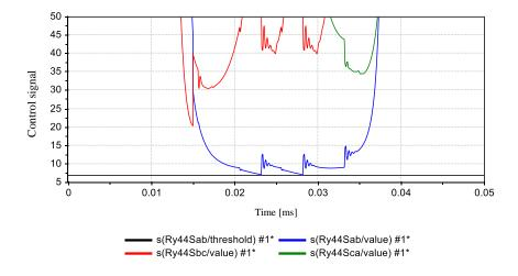
Figure 7 Calculated value of 44S at 0.5 cycle interruption (the black line is the settling value)
