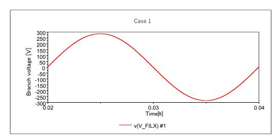
(a) AC voltage waveform at outlet of AC filter
