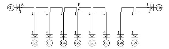
Figure 1 Benchmark power system model of the "WEST 10 System" of the Institute of Electrical Engineers
