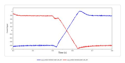
Figure 5 Active power [pu] Blue line, terminal 1; red line, terminal 2 the (reference capacitance is 55.9 MVA)
