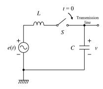
Figure 2 Equivalent circuit for energization of a no-load transmission line
