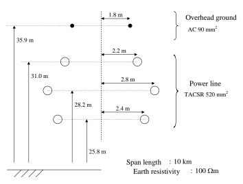
Figure 2 Poles of the 66-kV transmission line
