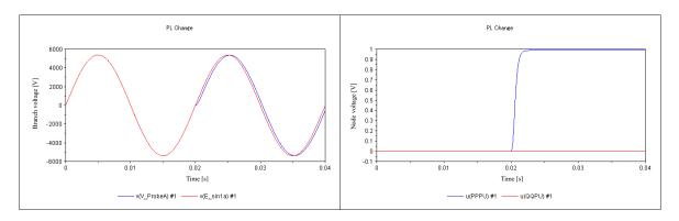
Phase A voltage [V] on the power and load sides
