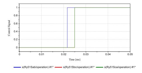
Figure 12 51S output at one cycle interruption
