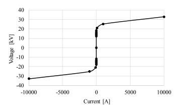
Figure 5 *V-I* characteristics of surge arrester.
