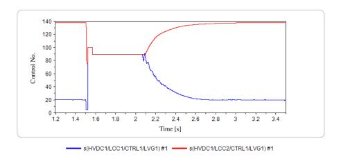
Figure 11 Control angle  $\alpha$  Red line, 50-Hz side; blue line, 60-Hz side
