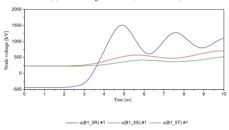
(c) Busbar voltage waveform (transformer end)
