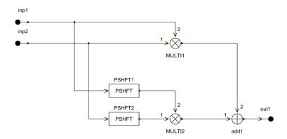
Figure 4 Phase difference calculation
