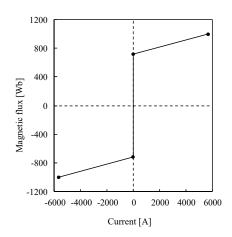
Figure 6 Saturation characteristics of excitation inductance
