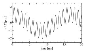
Figure 3 Voltage waveform when energizing a no-load transmission line (lumped constant capacitance approximation)
