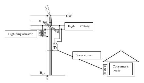
Figure 1 Conceptual diagram of lightning surge analysis from the secondary side of pole-mounted transformer
