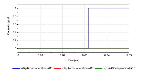
Figure 14 44S output at one cycle interruption
