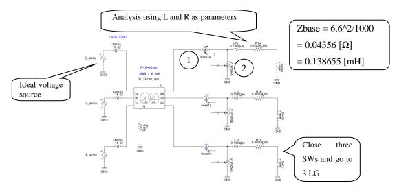
Figure 1 Analysis circuit
