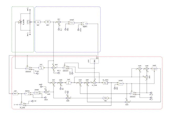
Figure 2 Implementation of the Motoyama model (simplified model)
