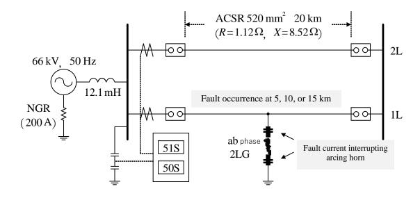
Figure 1 Single-line diagram of the model system
