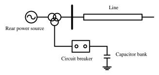
Figure 3 Illustration of capacitive current switching
