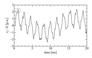
Figure 5 Remote-end voltage waveform when energizing a no-load transmission line (simulation using a no-loss distributed constant circuit)
