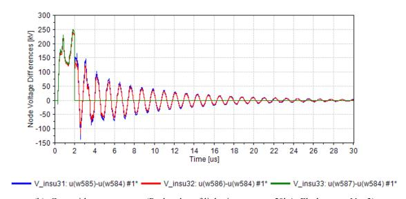
(b) Case with surge arrester (Peak value of lightning current: 50kA, Flashover at No. 3) Figure 9 Insulator voltage when the flashover occurs obtained by the triangular lightning current waveform.
