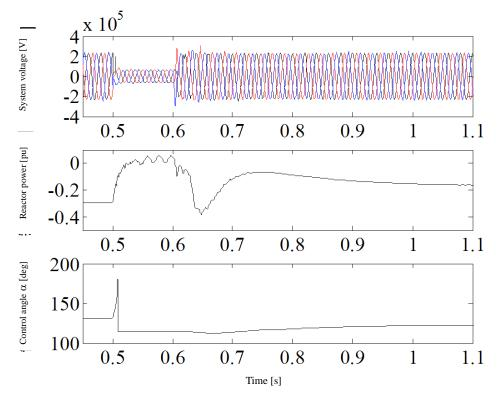
Figure 5 Waveform of each part at the time of three-wire ground fault
