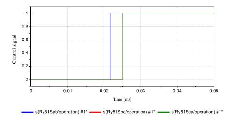
Figure 6 51S output at 0.5 cycle interruption
