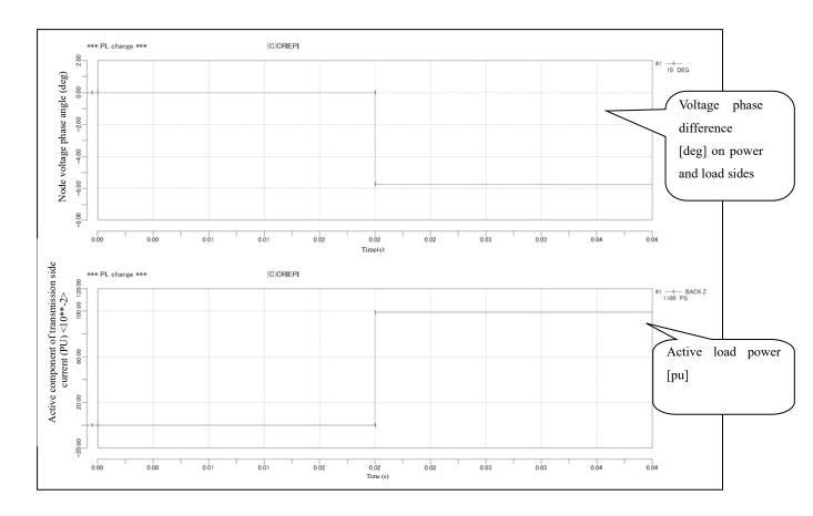
It can be seen that the load generates a phase difference in the voltage on the power supply and load sides. The change in the active power is clean owing to the resistive load.
