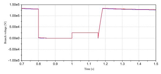
Figure 6 DC voltage [pu]: blue line, terminal 1; red line, terminal 2 (reference voltage of 125 kV)
