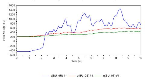
(b) Busbar voltage waveform (center of the bus)
