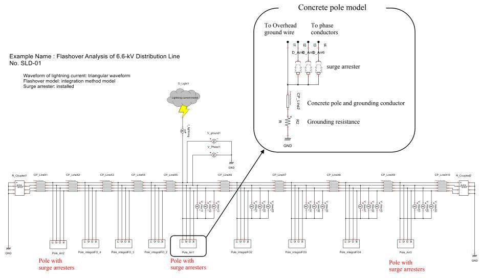
Figure 6 Overview of calculation model in XTAP.
