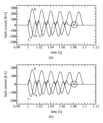
Figure 6 Ground fault current waveform at ground point J: (a) daytime and (b) nighttime sections
