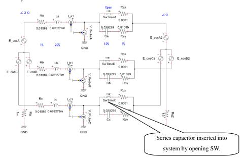
Figure 1 Analysis circuit
