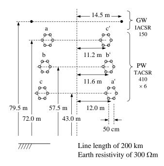
Figure 1 Pillar assembly of 500-kV vertically arranged double circuit transmission line
