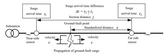
Fig. 1 Standardization principle of ground-fault surge arrival time difference analysis method
