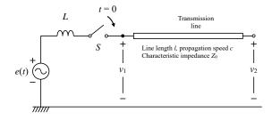
Figure 4 Equivalent circuit for energization of a no-load transmission line (simulation using a no-loss distributed constant circuit)
