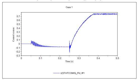
Figure 4 Reactive power output by STATCOM [pu]
