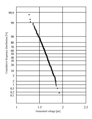
Figure 8 Cumulative frequency distribution of the voltages appearing in busbar 5
