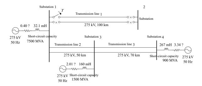
Figure 10 Example circuit for switching surge calculation
