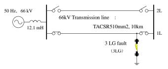
Figure 1 Single-line diagram of the model system
