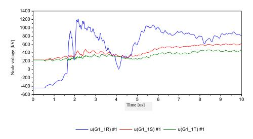
(a) Busbar voltage waveform (substation entrance)
