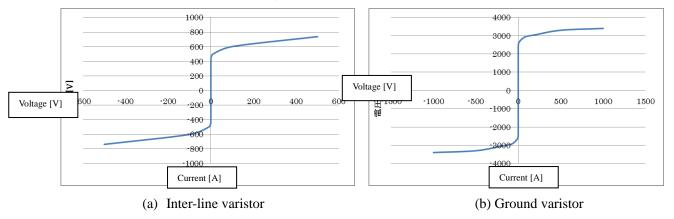
Figure 5 Example of the V-I characteristics of varistor used in consumer equipment
