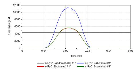
Figure 5 51S calculation value at 0.5 cycle interruption (the black line is the settling value)
