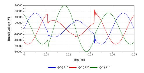
Figure 10 Voltage waveform at one cycle interruption
