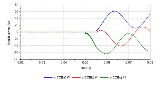
Figure 9 TRV waveform at the time of capacitive current switching
