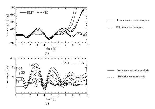
Figure 5 Comparison of the results of instantaneous value analysis using XTAP and effective value analysis using CPAT
