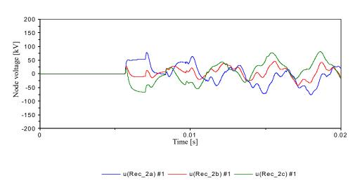
(c) 2L Remote-end voltage waveform
