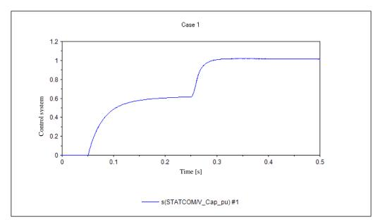
Figure 3 Capacitor voltage for energy storage [pu]
