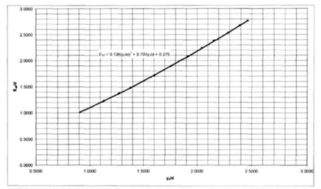
FIGURE 9.11: Relationship between stage (y<sub>2</sub>) and energy level in pool (Es<sub>5</sub>) for d/b=0.5 with Crump weir
