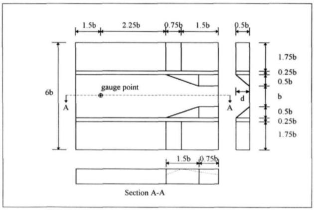
FIGURE 1.1:- Sluicing flume from previous study (WRC,1995)
