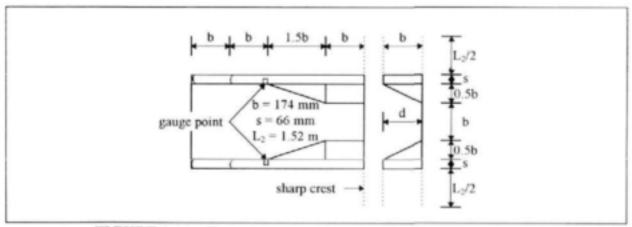
FIGURE 9.14: Flume lay-out - b/d=1.0 with sharp-crested weir
