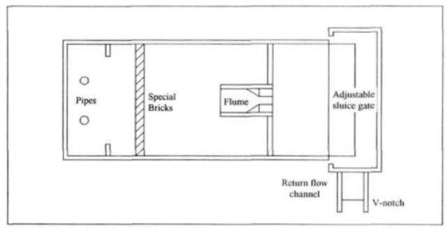
FIGURE 4.2 - Schematic diagram of channel in which model studies were undertaken
