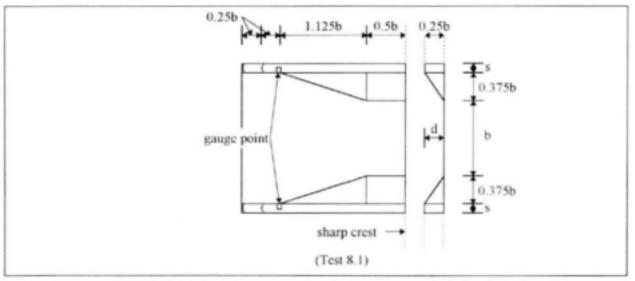
FIGURE 4.12 - Dimensions for flume lay-out 3S (d/b =0.25)
