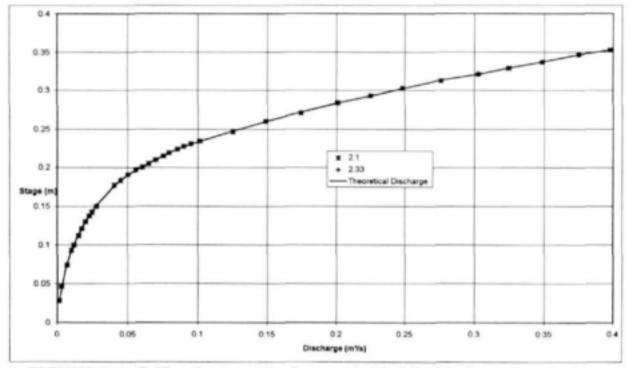
FIGURE 9.18: Calibration curve for flume with d/b=1.0 with sharp-crested weir as tested in model
