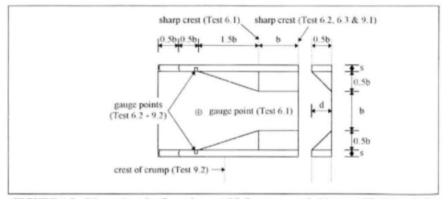
FIGURE 4.7 - Dimensions for flume lay-out 2S & recommended lay-out 2R (d/b = 0.,5)
