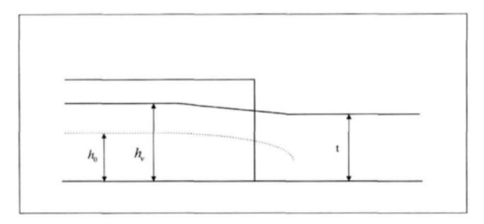
FIGURE 7.1 - Definition sketch of submerged conditions for flow in flume
