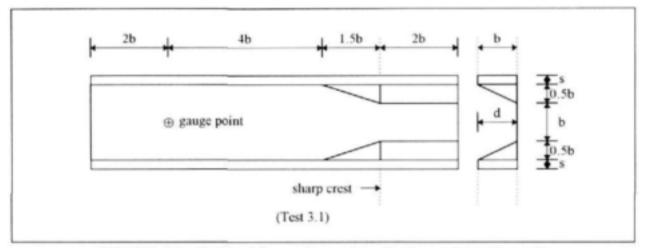
FIGURE 4.8 - Original flume dimensions for lay-out 1 (d/b = 1.0)
