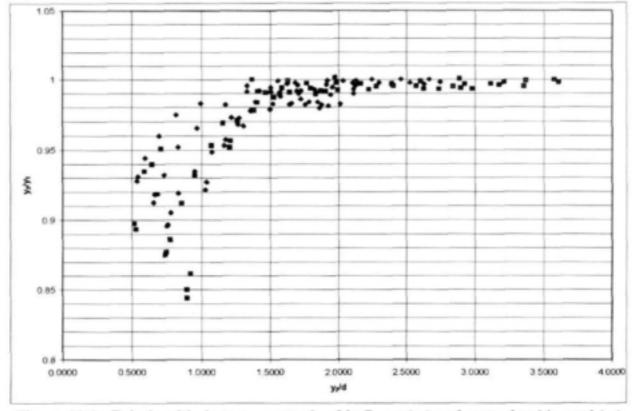
Figure 10.6: Relationship between water level in flume (y<sub>2</sub>) and water level in pool (y<sub>5</sub>) under non-modular conditions for flume combined with sharp-crested weirs.
