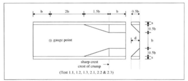
FIGURE 4.5 - Original flume dimensions for lay-out 2 (d/b = 0.5)
