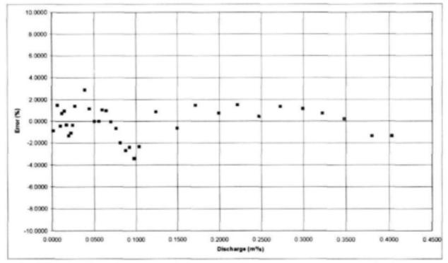
FIGURE 9.19: Error in derived discharge relative to measured discharge for flume with d/b=1.0 with sharp-crested weir
