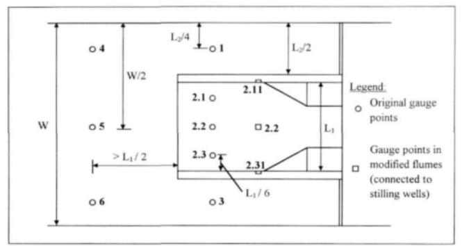
FIGURE 4.3 - Lay-out showing positions of gauge points
