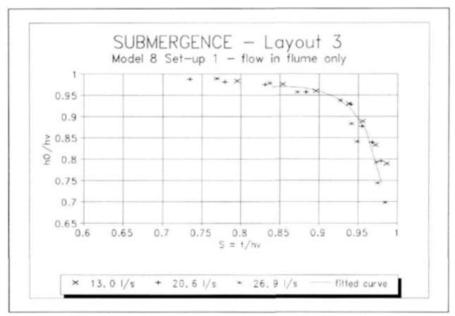
Figure 7.10 - Submergence in model lay-out 3S for flows in flume
