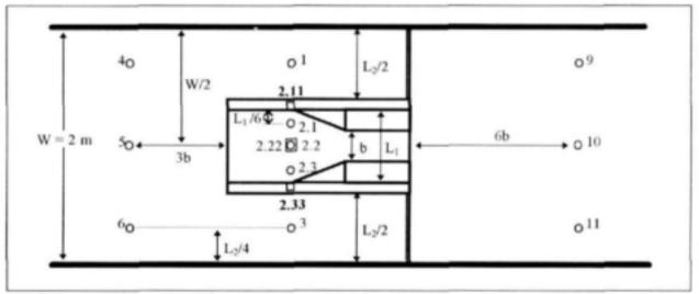
FIGURE 9.1: Water level recording positions
