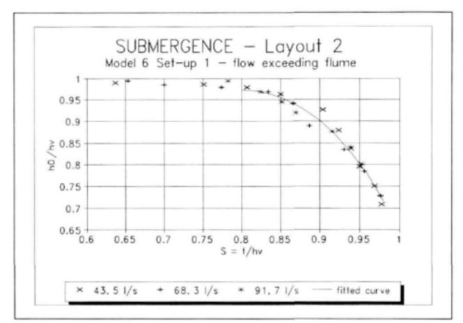
FIGURE 7.9 - Submergence in flume lay-out 2S for flows exceeding flume capacity
