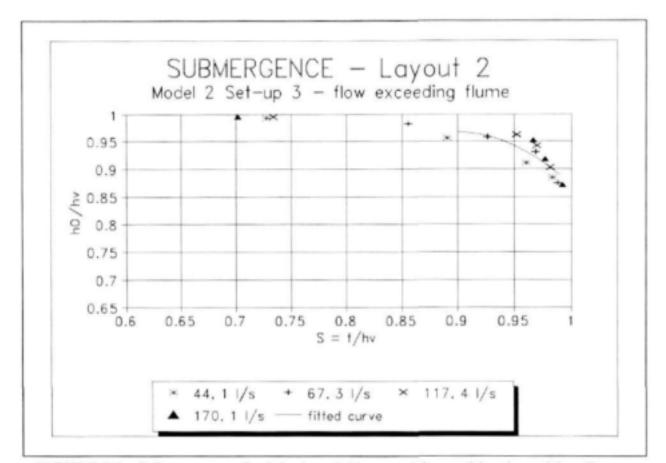
FIGURE 7.5 - Submergence of original model lay-out 2 in combination with a Crump weir
