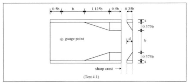
FIGURE 4.11 - Original flume dimensions for lay-out 3 (d/b = 0.25)
