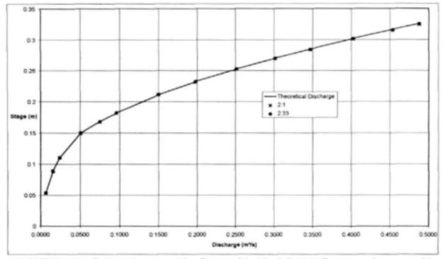
FIGURE 9.12: Calibration curve for flume with d/b=0.5 with Crump weir as tested in model
