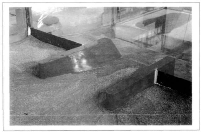
FIGURE 6.4 - Siltation of flume under conditions of low discharge
