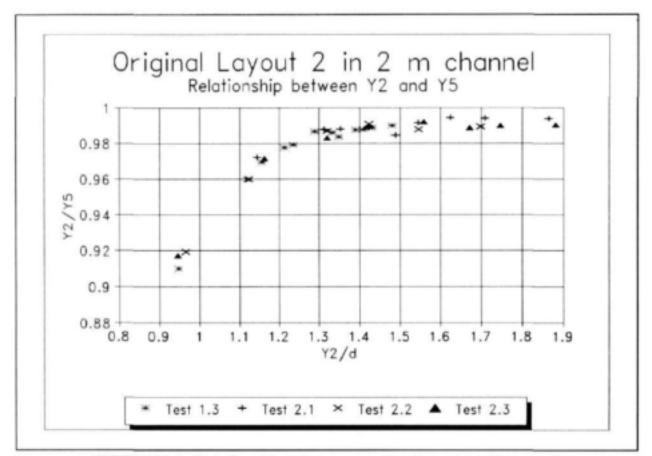
FIGURE 5.6 - Relationship between y2 and y5 for original lay-out 2
