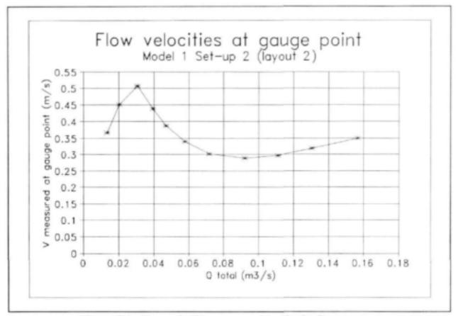
Figure 5.4 - Flow velocities measured inside the flume
