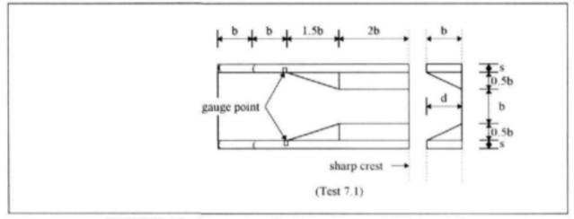
FIGURE 4.9 - Dimensions for flume lay-out 1S (d/b = 1.0)
