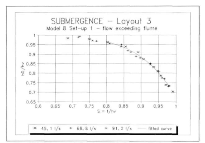
Figure 7.11 - Submergence in flume lay-out 3S for flows exceeding flume capacity
