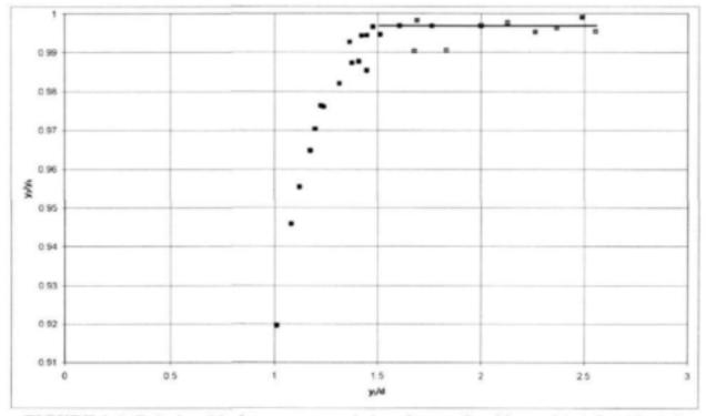
FIGURE 9.4: Relationship between stage (y<sub>2</sub>) and water level in pool (y<sub>5</sub>) for d/b=0.5 with sharp-crested weir
