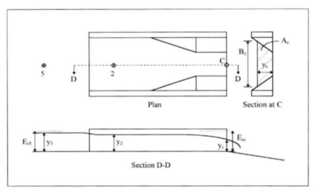
FIGURE 3.1: Definition sketch - flow in flume only
