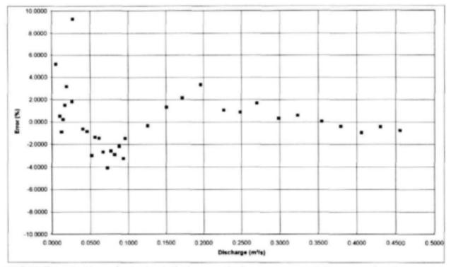
FIGURE 9.25: Error in derived discharge relative to measured discharge for flume with d/b=0.25 with sharp-crested weir
