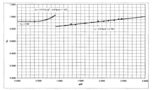
FIGURE 9.9: Discharge coefficients for flume with d/b=0.5 in combination with a Crump weir.
