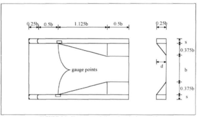
FIGURE 5.2 - New proposed dimensions for lay-out 3S
