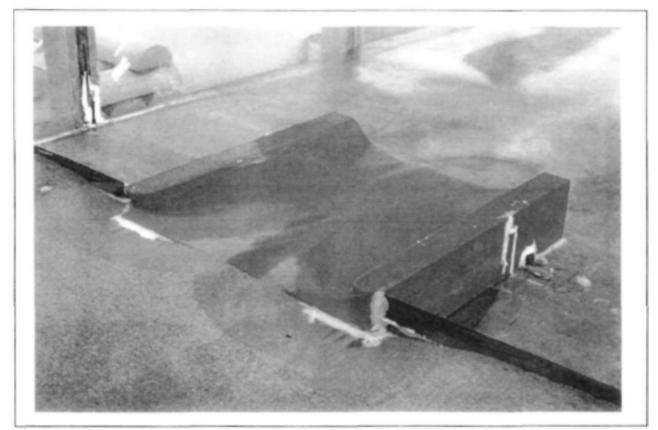
FIGURE 6.5 - Flume with new weir position
