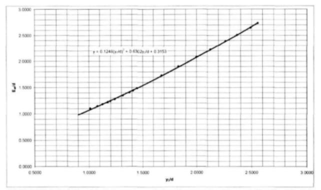
FIGURE 9.5: Relationship between stage (y<sub>2</sub>) and energy level in pool (E<sub>s5</sub>) for d/b=0.5 with sharp-crested weir
