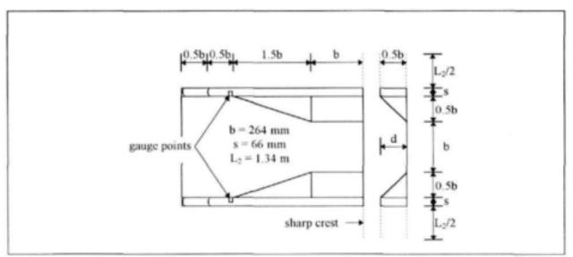
FIGURE 9.2: Flume lay-out - b/d=0.5 with sharp-crested weir
