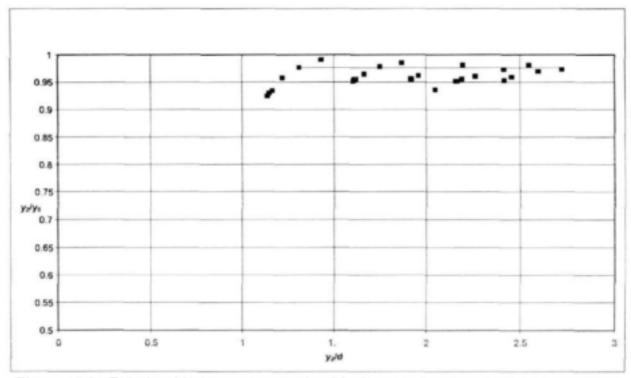
Figure 10.8: Relationship between water level in flume  $(y_2)$  and water level in pool  $(y_5)$  under non-modular conditions for flume combined with a Crump weir (d/b = 0.5).
