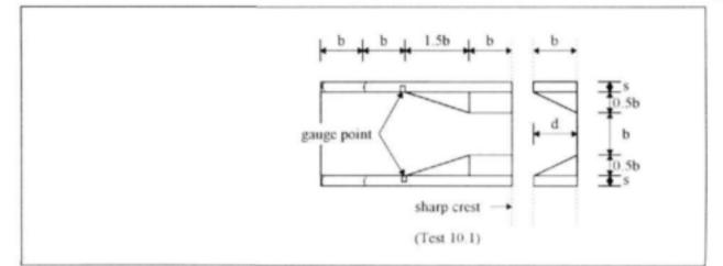
FIGURE 4.10 - Dimensions for recommended flume lay-out 1R (d/b = 1.0)
