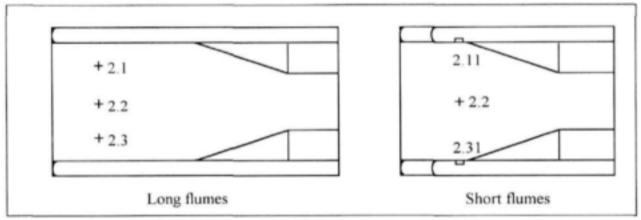
FIGURE 5.1 - Positions for stage measurement in flumes
