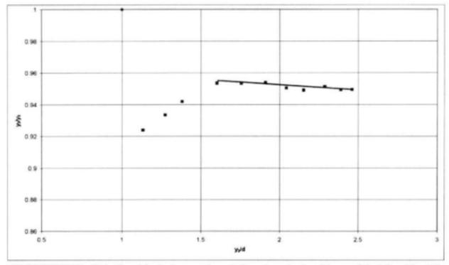
FIGURE 9.10: Relationship between stage (y<sub>2</sub>) and water level in pool (y<sub>5</sub>) for d/b=0.5 with Crump weir
