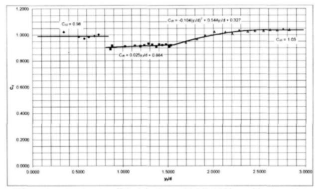
FIGURE 9.21: Discharge coefficients for flume with b/d=0.25 in combination with a sharp-crested weir
