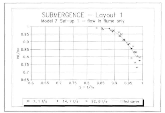
Figure 7.6 shows submergence properties of the adapted model lay-out 1, for discharges not exceeding flume capacity, with a curve fitted to submergence levels exceeding 80 %.
