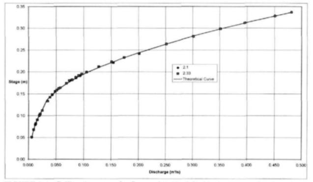
FIGURE 9.6: Calibration curve for flume with d/b=0.5 with sharp crested weir as tested in the model
