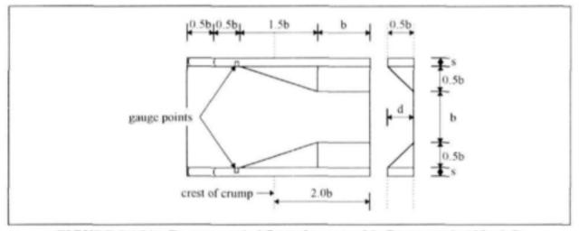
FIGURE 8.1(b): Recommended flume lay-out with Crump weir (d/b=0.5)
