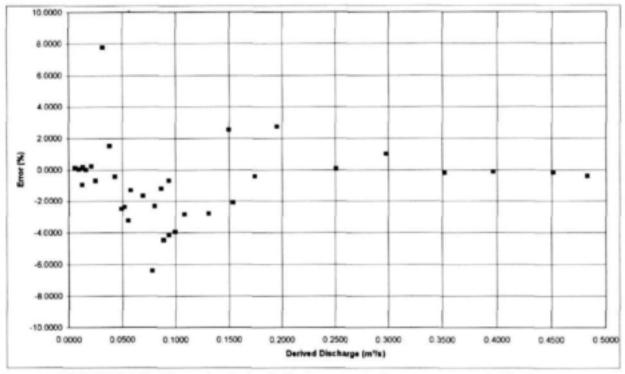
FIGURE 9.7: Error in derived discharge relative to measured discharge
