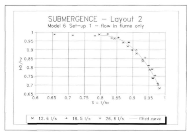
FIGURE 7.8 - Submergence in model lay-out 2S for flows in flume
