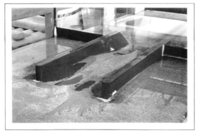
FIGURE 6.2 - Sediment accumulated in parallel-wall section
