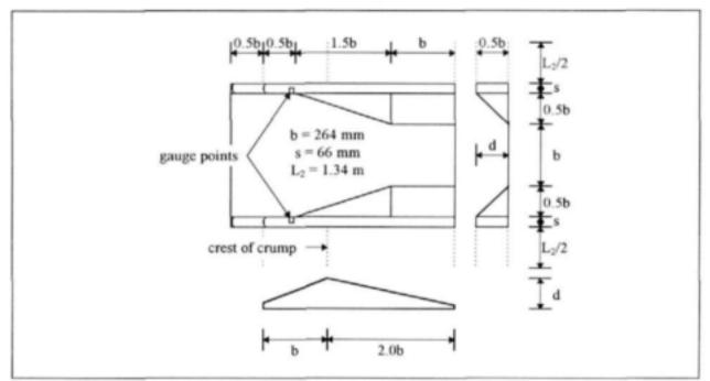
FIGURE 9.8: Flume lay-out - b/d=0.5 with Crump weir
