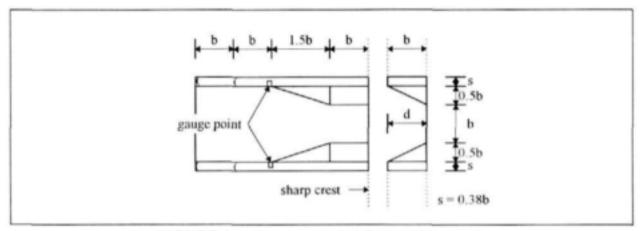
FIGURE 8.2: Recommended flume with d/b=1
