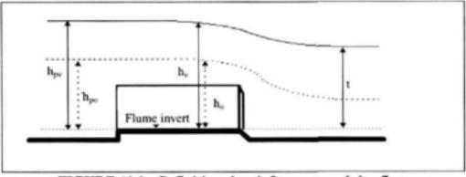
FIGURE 10.2: Definition sketch for non-modular flow
