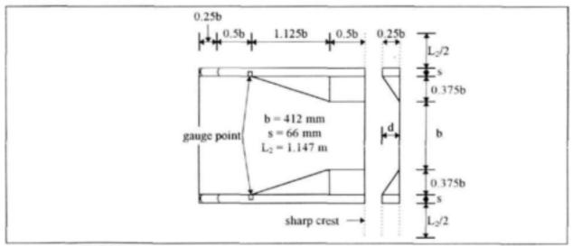
FIGURE 9.20: Flume lay-out - b/d=0.25 with sharp-crested weir
