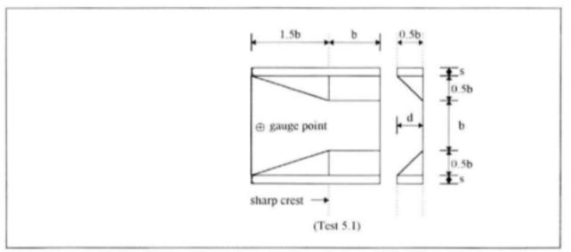
FIGURE 4.6 - Dimensions for flume lay-out 2VS (d/b = 0.5)
