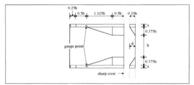
FIGURE 8.3: Recommended flume for d/b= 0.25
