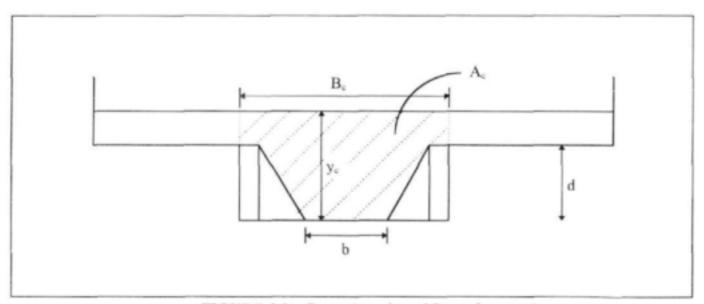
FIGURE 3.2: Control section of flume for  $y_c > d$
