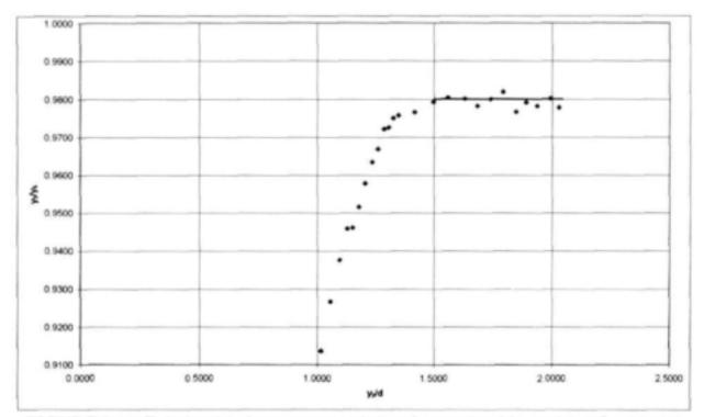
FIGURE 9.16: Relationship between stage (y<sub>2</sub>) and water level in pool (y<sub>5</sub>) for d/b=1.0 with sharp-crested weir
