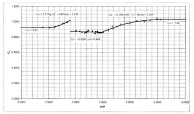
FIGURE 9.3: Discharge coefficients for flume with b/d=0.5 in combination with a sharp-crested weir
