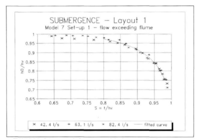
FIGURE 7.7 - Submergence in flume lay-out 1S for flows exceeding flume capacity
