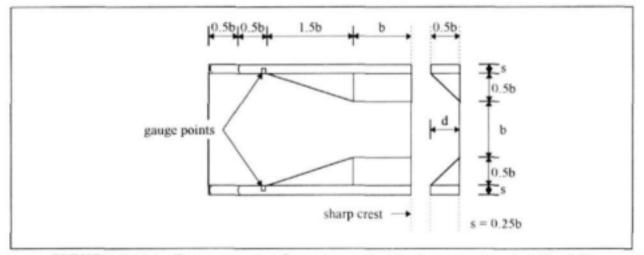
FIGURE 8.1(a): Recommended flume lay-out with sharp crest weir (d/b=0.5)
