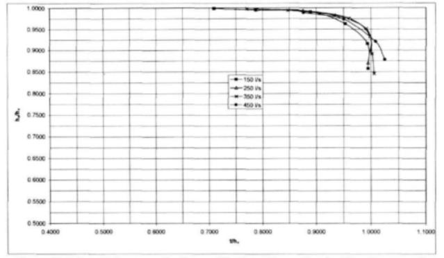
Figure 10.7: S vs. h<sub>0</sub>/h<sub>v</sub> curves for flume with d/b = 0.5 combined with a Crump weir
