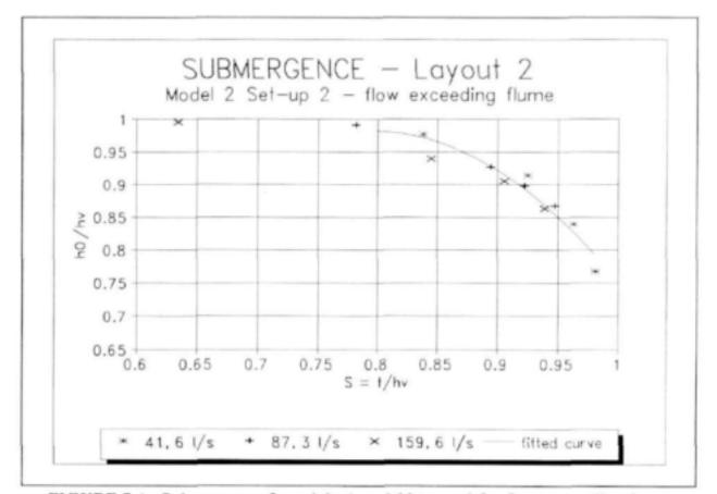
FIGURE 7.4 - Submergence for original model lay-out 2 for flows exceeding flume capacity
