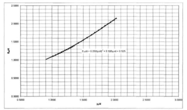
FIGURE 9.17: Relationship between stage (y<sub>2</sub>) and energy level in pool (Es<sub>5</sub>) for d/b=1.0 with sharp-crested weir
