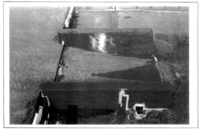
FIGURE 6.7 - Sedimentation in flume with low step in mouth
