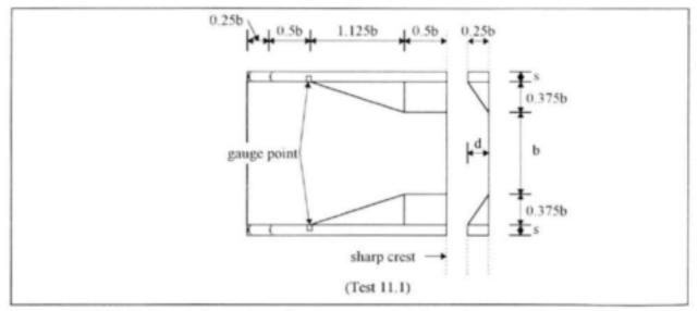
FIGURE 4.13 - Dimensions for recommended flume lay-out 3R (d/b =0.25)
