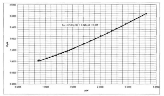
FIGURE 9.23: Relationship between stage (y<sub>2</sub>) and energy level in pool (Es<sub>5</sub>) for d/b=0.25 with sharp-crested weir
