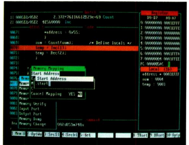
Fig. 3. Memory mapping of target to emulator in Sigma package allows emulator to behave exactly as target hardware.
