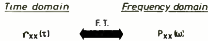
Fig. 7.4. Wiener-Khinchine theorem relates autocorrelation function in time domain and power spectral density function in frequency domain as a Fourier transform pair.
