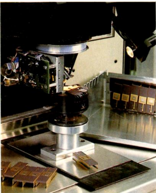
Two packaging operations at Iteq: bonding wires to a 40-lead side-braze package (above), and sealing pin-grid arrays (top right).
