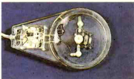
Pulsed series oscillator. Coil diameter is 70mm. The negative resistance/voltage limiter is built as a thick-film hybrid micro-circuit on a substrate measuring 25mm square.
