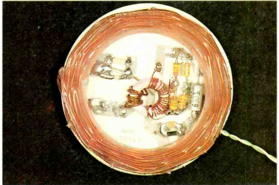
Implantable receiver, also in thick-film before encapsulation in silicone rubber. Diameter is 43mm. Used with the oscillator shown left, the receiver delivers 30V into 390 ohms.
