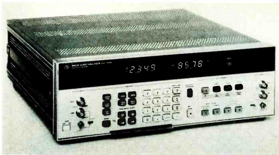
With a personal computer, some software and a few t.t.l. i.c.s, the 8903A audio analyser becomes an audio test station.
