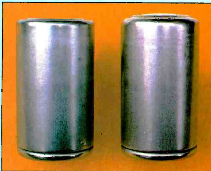
Fig. 7. An overcharged cell showing a bulge in the base caused by high internal pressure prior to the safety vent opening. A normal cell is shown for comparison. A condition like this is a sure sign of abuse, whether due to charging at too low a temperature, reverse charging or to charging in excess of C/10.
