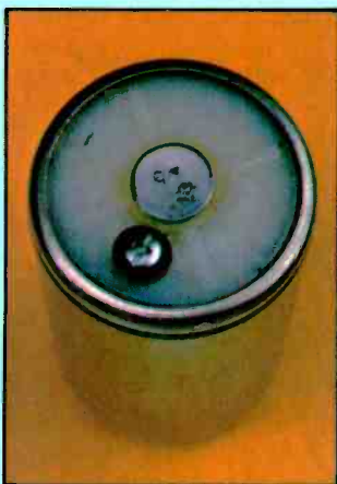
Fig. 8. A cell which has "dried out", modified by putting a filler hole in the top so that water can be introduced in controlled quantities. The filler hole in this particular cell is sealed with a nickel-plated steel pan-head M2.5 screw, which does not interfere with normal use of the cell. A small neoprene washer completes the seal.
