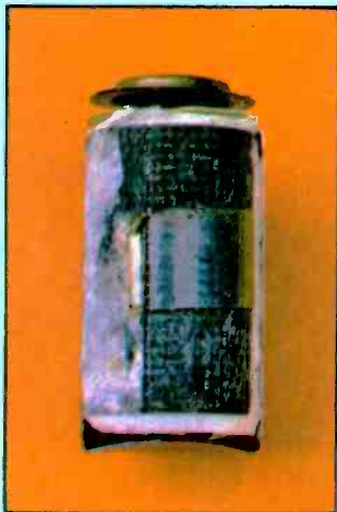
Fig. 6. An overcharged cell, sectioned to show the collapsed base. This cell was overcharged due to a fault in the charger, but shows what can happen when any cell is charged for longer than is necessary at a rate which is too high. The contents of this cell were expelled when the cell became hot, and on cooling the case collapsed inward.
