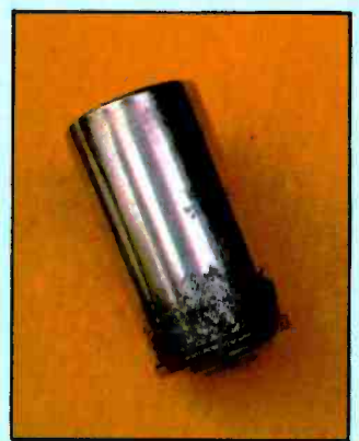
Fig. 11. Localised pin-hole corrosion caused in this instance by contact with sea water for a short time. This also could have been prevented by grease or paint.
