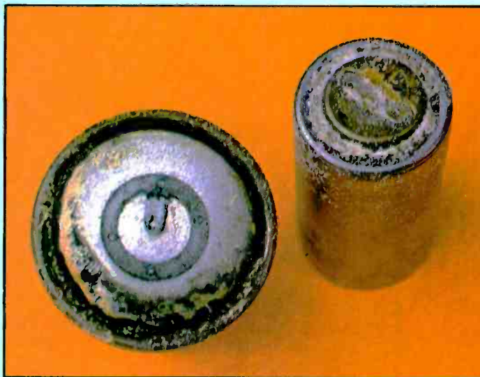
Fig. 9. The effects of electrolyte creepage on two types of cell. The deposit has started to corrode the cell on the left.
