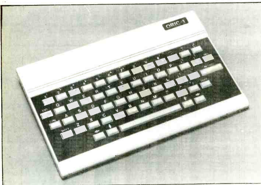
"Some manufacturers have the u.l.a. made for them to the specification of the computer," says Oric computer designer P. T. Johnson of Tangerine Computer Systems, "rather than designing the u.l.a. around it". Like many popular computers Oric 1 is based on a 6502 microprocessor and a u.l.a., but unlike others it provides an eight-colour facility together with 15K of user ram for £100. A printer and disc drive are promised for the near future, as is a £60 modem to interface with videotex systems.
