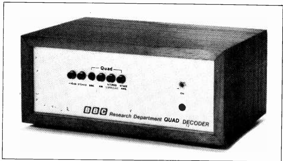
Early laboratory model of Matrix H decoder developed at BBC
