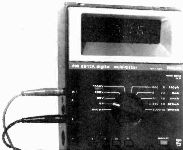
PM2513A New 3\frac{1}{2} -digit Battery operated dmm with 11mm LED display
