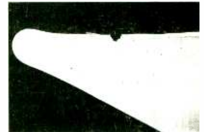
Sectioned iron-plated bit, after 40,000 simulated operations using SAVBIT Solder.
