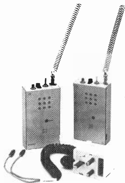
General view of the pair of two-metre transceivers ready for use. Also shown is the mains battery-charging unit which plugs directly into a 13 amp power point.
