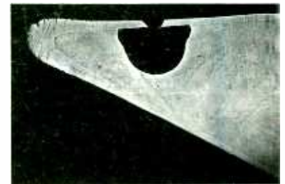
Sectioned iron-plated bit, after 40,000 simulated operations using 60/40 Solder.
