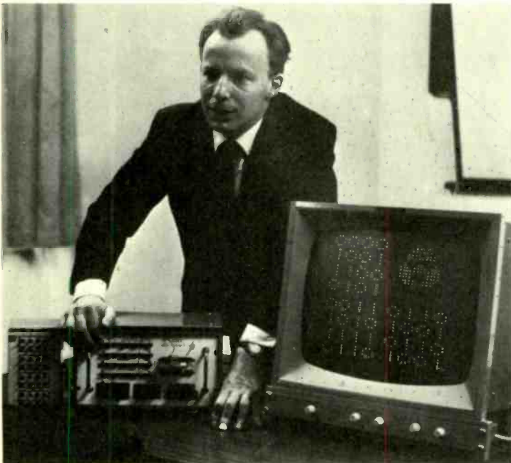
At the invitation of the British Computer Society, Brian Crank, the designer, described the "Wireless World" Logic Display Aid at a meeting of the Logic Design Group on July 9th: a 19-inch oscilloscope made by Lan Electronics was used for the demonstration.
