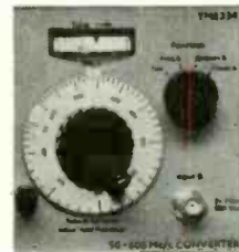
TM 8334 extends frequency to 600 MHz.
