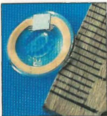
Lens incorporating a chip, pressure sensor and RF coil, provides early warning of pressure build-up in the eye, and 24-hour monitoring.
