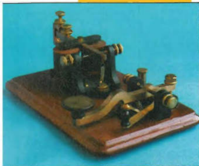
typical KOB - key on base. This includes a camelback key and sounder. This example was made around 1860.
