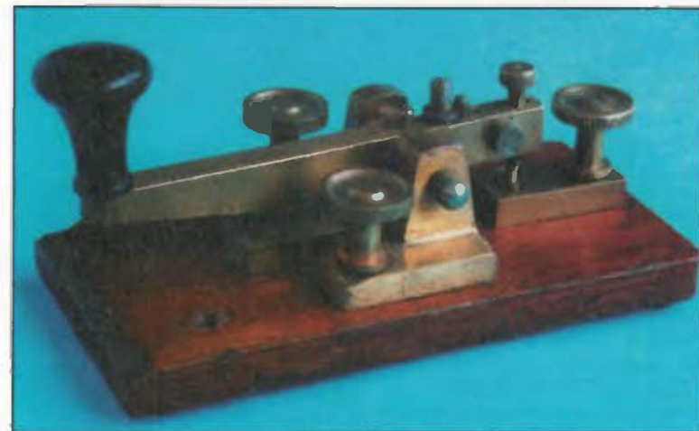
A key used by the British Post Office. Note the heavy brass construction. This key was manufactured around 1900.
