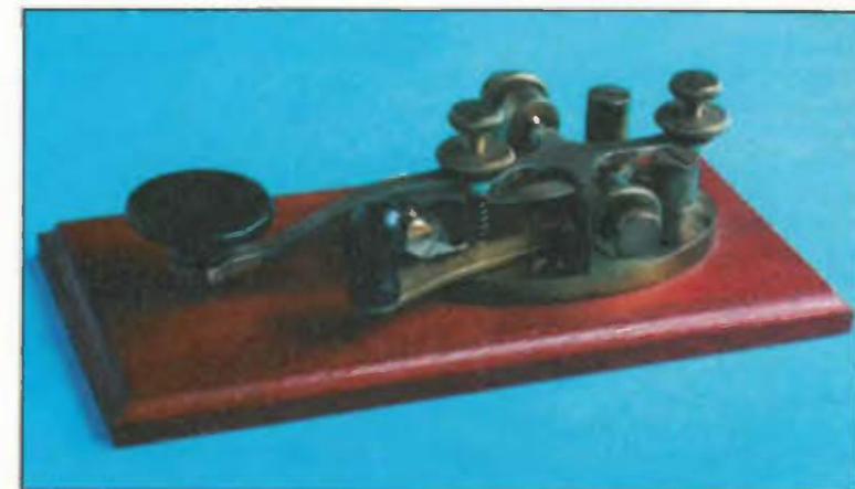
A steel lever key. This particular example was manufactured in the USA around 1920.
