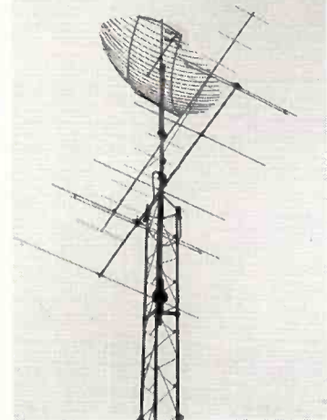
Fig. 2: A selection of antennas used by Roger Bunney during the early Seventies. Note the u.h.f. antenna with a 2m parabolic reflector!
