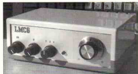
Fig. 3: An example of tuning simplicity: an outboard v.h.f./u.h.f. tuner with simple rotary tuning knob.
