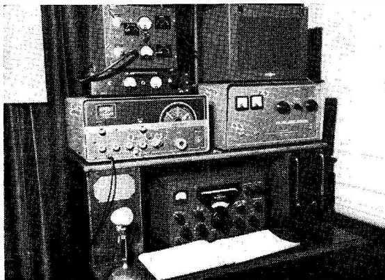
Station G3JNY, run by Sam Ellis at 2 St. Mary's Close, Garforth, Leeds, Yorkshire, with a nice array of gear. The main Rx is a Collins 75A, with a BRT-400 as stand-by. On the transmitting side, a Hallicrafters HT-37 drives a KW-500 linear for multi-band working, for which a Joystick is used, tuned by a Minimitter ATU. In addition, he has two TW Communicators, one for Top Band and the other for two metres, for which the beam is a 6-over-6. Now in the Radio/TV business, Sam has been interested in radio since the days of Kaiser's War surplus, having started with crystal receivers and one-valve sets. For him, G3JNY is nowadays just a relaxing hobby, indulged in when the spirit moves and the urge for DX stirs him into activity.
