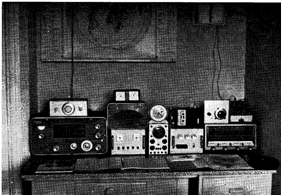
Fine array of equipment owned by Stuart Ralph, 59 Church Road, Earley, Reading, Berks., who has been an SWL for about ten years. His main Rx (left) is a Minimitter MR44/II, with a Codar PR-30X preselector above it; next is a home-built PSU and then a Heathkit OS-1 'scope, used mainly in conjunction with the receiver. The other gear includes a 12w. transistor amplifier, a tape recorder, and a Hallicrafters S.38E, used for general-coverage listening and also as IF/AF strip for VHF converters for two and four metres. His aerials consist of dipoles in the roof space. Stuart remarks that his "main interests are SSB on 15-20-80m., with occasional CW listening on these bands."
