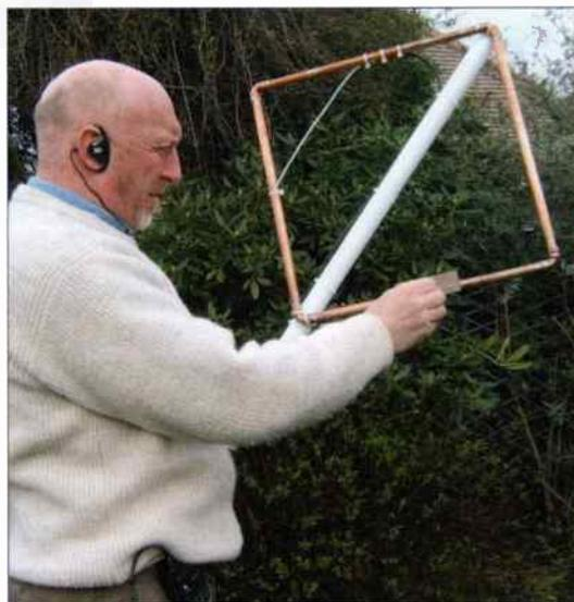
The antenna can be connected directly to 50Ω coaxial cable, with the outer connected to a point directly opposite the tuning capacitor, and the inner to a point half way along one of the other sides. I fixed a solder tag to the copper pipe and soldered the coaxial outer to that, to minimise the heat
