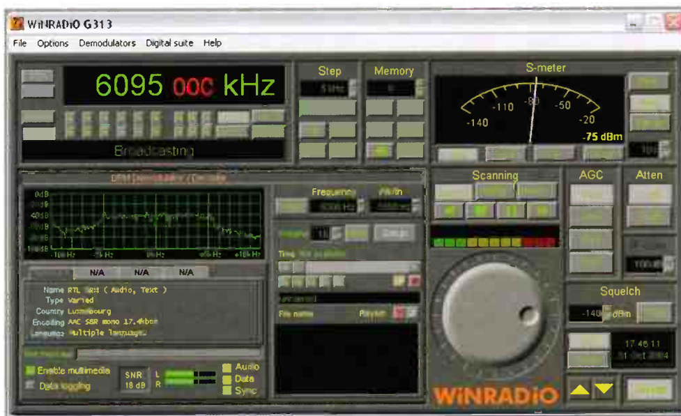
● The DRM Demodulator plug-in appears as an integral part of the main panel with its own real-time bandscope and recorder. Transmission data and scrolling text appear below the bandscope.
