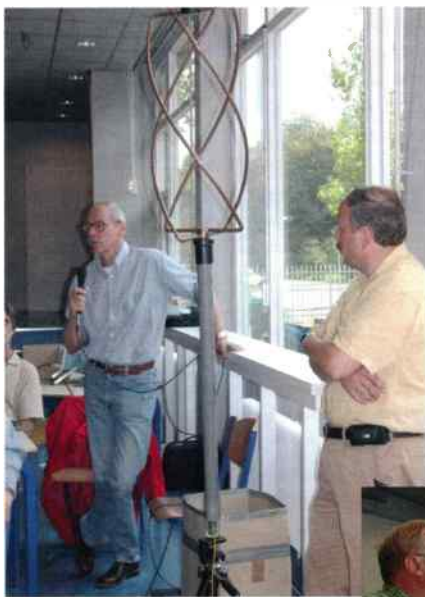
● Fig. 3: Rob Hollander explaining the QFH antenna used for a.p.t. reception.
