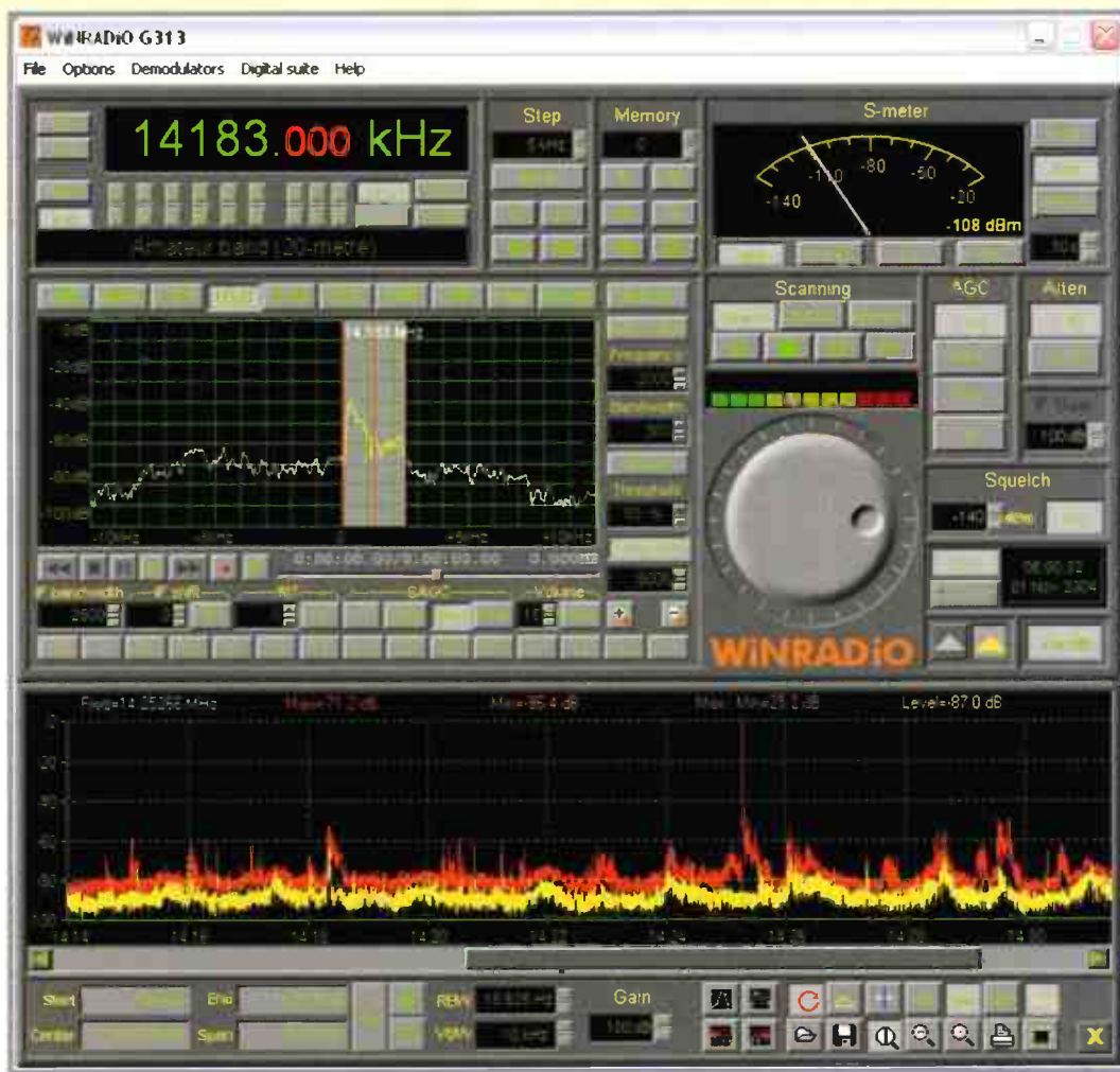
● The spectrum analyser showing part of the 20m amateur band with average (yellow) and maximum (red) levels as recorded over the course of one minute.
