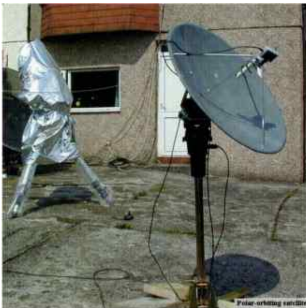
Fig. 1: METEOSAT PDUS dish near the house, telescope under cover, new tracking dish. The house is near due east and cuts off passes below 60° elevation!
