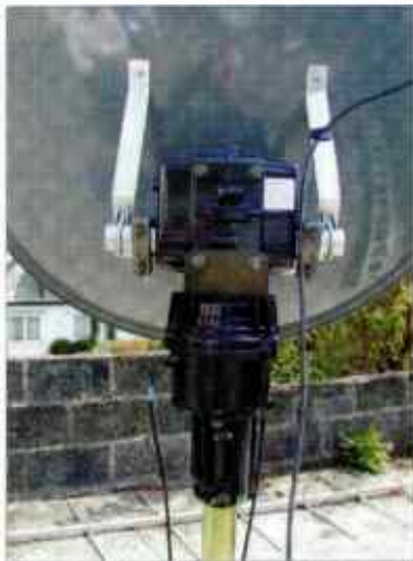
Fig. 3: Close-up of rear of dish and support brackets.
