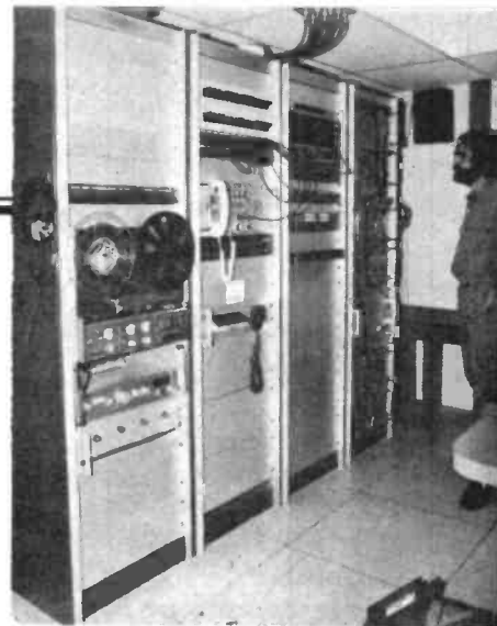
Radio Avui in Barcelona, HQ station of the Cadena 13. Note the tape recorder for off-air logging
