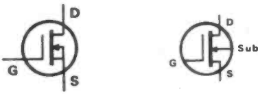
Fig 1 Symbols of 3-pin and 4-pin n-channel depletion mode MOSFETs
