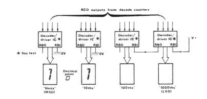
Fig 8 Trailing zero suppression in a 31/2-digit DVM readout
