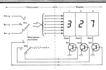
Fig 3 Method of multiplexing a 3-digit common-cathode LED display
