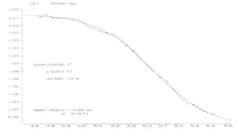
Fig 5 Doppler frequency plot for cosmos navigation satellite
