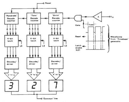
Fig 2 Improved digital 'frequency' meter circuit
