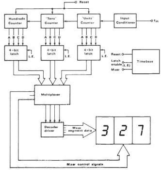
Fig 4 Realistic implementation of the multiplexing technique in a 3-digit frequency meter
