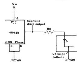
Fig 22 Driving a commoncathode LED display with a 4543B
