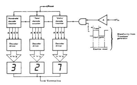
Fig 1 Simple digital 'frequency' meter circuit
