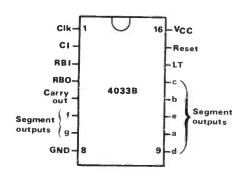
Fig 28 Pin designations of the 4033B decade counter with 7-segment outputs and ripple blanking
