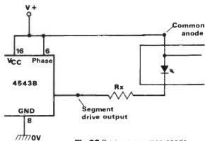
Fig 23 Driving a common-anode LED display with a 4543B
