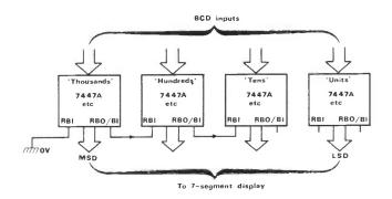
Fig 13 Method of applying leading-zero suppression to the first three digits of a 4-digit display, using the '7447A' family of ICs
