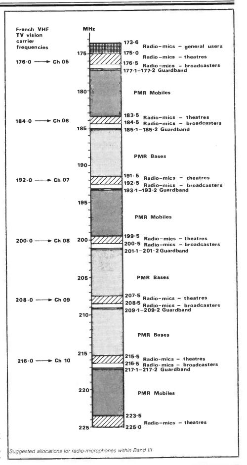
services in Band III. The proposed bandplanning for the re-use of Band III has therefore avoided the vision carrier frequencies of Canal Plus. These frequencies will be allocated to services that would not be so susceptible to interference from overseas TV transmitters
