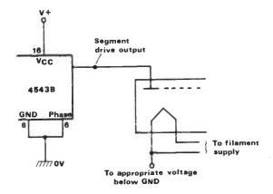
Fig 25 Driving a flourescent readout with a 4543B
