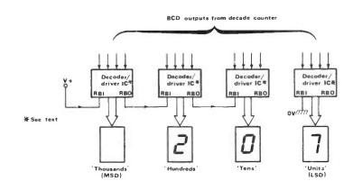
Fig 7 Leading zero suppression in a 4-digit counter
