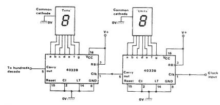
Fig 29 Basic method of cascading 4033B ICs (without zero suppression)
