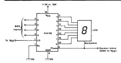
Fig 21 Using the 4543B to drive a
