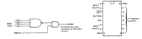
Fig 9 DIY 'ripple blanking' logic (active high type)
