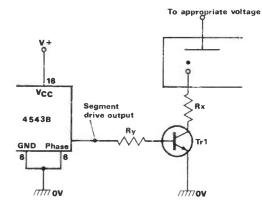
Fig 24 Driving a gas-discharge readout with a 4543B
