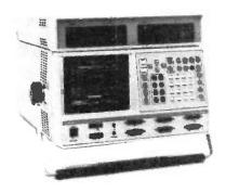
The K205's tolerance compare feature allows fast analysis of logic circuits by comparing timing sequences against stored references. This facility eliminates sampling error difference inherent in asynchronous analysis. Reference data can be stored automatically via an input/output port, by testing a known good circuit, or by testing a known bad circuit, and manually editing a correct pattern.
