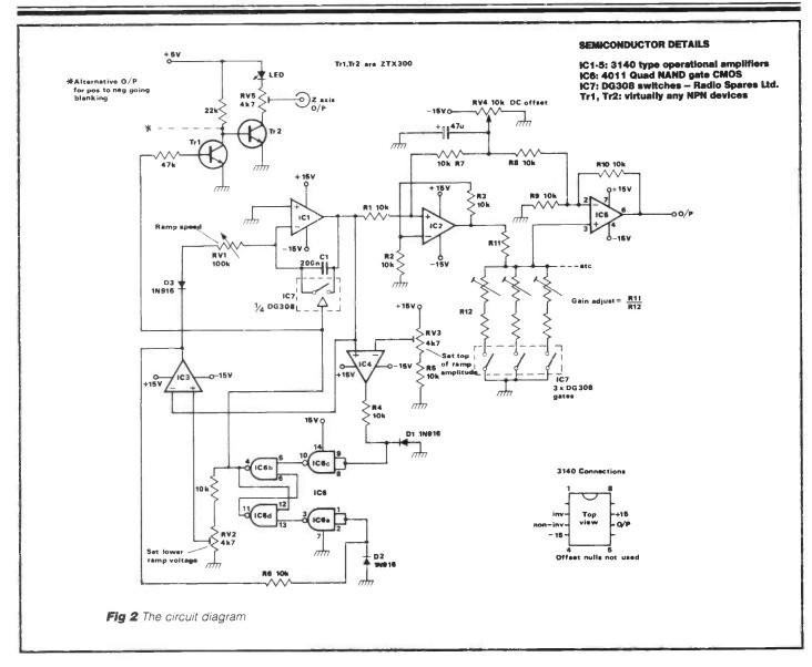
For Z-axis blanking two transistors, Tr1 and Tr2, provide a buffered drive which may be adjusted with RV5.
