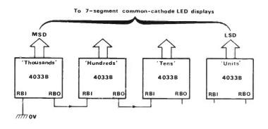
Fig 30 Method of modifying the Figure 29 circuit to give automatic leading-zero suppression
