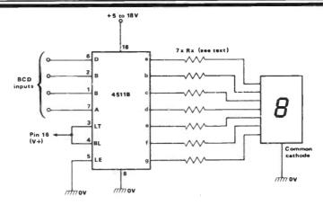
Fig 16 Using the 4511B to drive a common-cathode display
