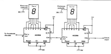
Fig 27 Basic method of cascading 4026B ICs
