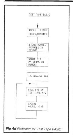
The program now transmits the time as three 6-bit bytes and two sub-routines, called 'GETBYTE' and 'TXBYTE' as described in the next sub-section.
