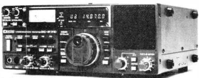
The R-70 also has separate antenna sockets for LW-MW with automatic switching, and a large, front-mounted loudspeaker with 5.8W output. The frequency stability for the 1st hour is  $\pm$  50Hz, sensitivity – SSB/CW/RTTY better than 0.32 uv for 12dB (S + N)  $\div$  N, Am – 0.5 uv. FM better than 0.32 for 12dB Sinad. DC is optional.
