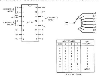
Fig 8 The 4051B 8-channel multiplexer/demultiplexer acts as single-pole 8-way switch
