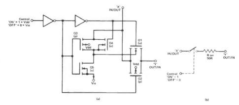
Fig 2 Basic circuit (a) and equivalent circuit (b) of the improved CMOS bilateral switch
