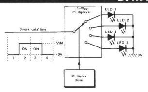
Fig 5 A 4-way multiplexer used to control four LEDs via a single DATA line
