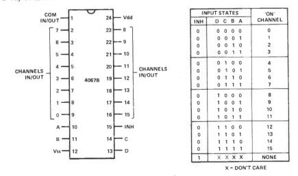
Fig 11 The 4067B 16-channel multiplexer/demultiplexer acts as a single-pole 16-way switch
