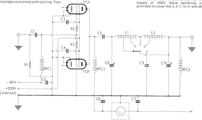
Fig 1 Circuit diagram 200W amplifier
