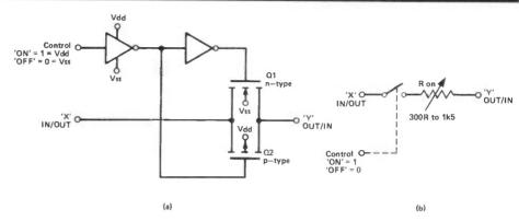
Fig 1 Basic circuit (a) and equivalent circuit (b) of the simple CMOS bilateral switch.
