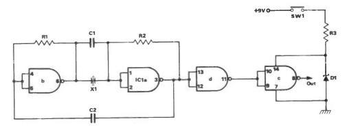
Fig 1a Crystal oscillator circuit
