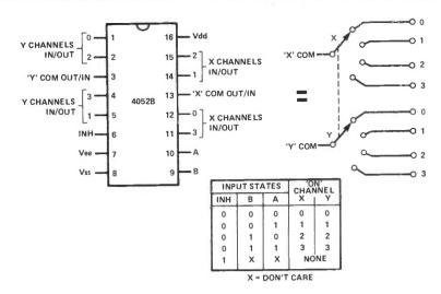
Fig 9 The 4052B differential 4-channel multiplexer/demultiplexer acts as a ganged 2-pole 4-way switch
