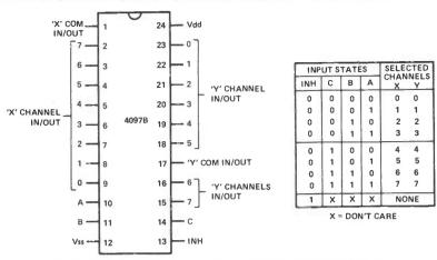
Fig 12 The 4097B differential 8-channel multiplexer/demultiplexer acts as a 2-pole ganged 8-way switch
