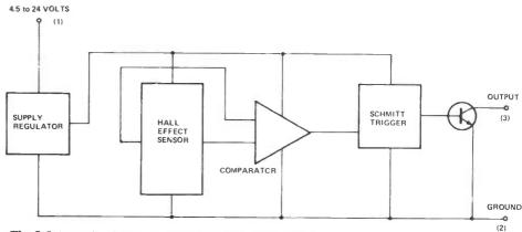
Fig 2 Schematic of Sprague 3020-type Hall effect switch
