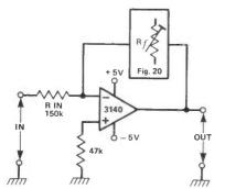
Fig 23 Digital control of gain, using the Fig 20 circuit. Gain is variable from zero to unity in 16 steps
