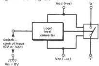
Fig 4 Some ICs feature internal 'logic level conversion', enabling an analogue switch to be controlled via a single-ended input
