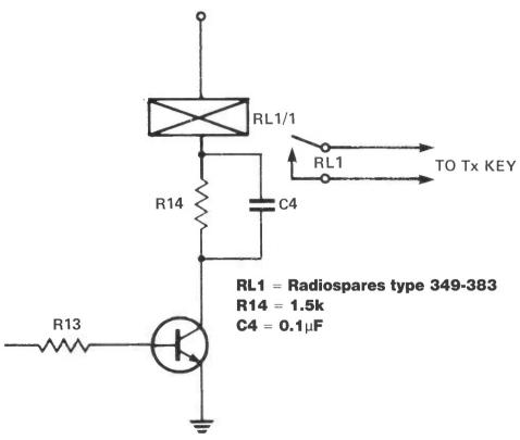
Fig 4 Alternative keying circuit using relay
