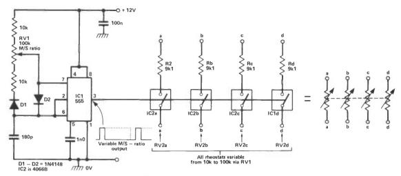
Fig 27 Synthesised precision 4-gang 'rheostat'
