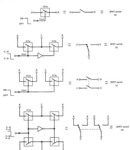
Fig 14 Implementation of the four basic switching functions via the 4066B (ICI)
