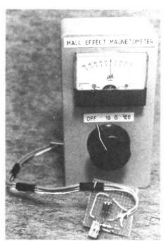
Hall effect Magnetometer with sensor mounted on bare board in front of main unit
