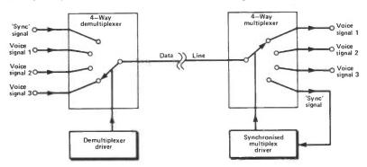
Fig 6 A 4-way multiplexer/demultiplexer combination used to feed three independent voice signals through a single DATA line
