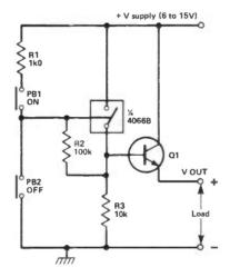
Fig 18 Latching push-button power switch
