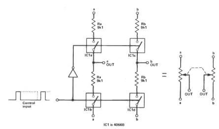
Fig 28 Synthesised precision 2-gang 'pot'
