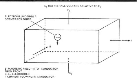
Fig 1 Schematic of Hall effect on current-carrying conductor
