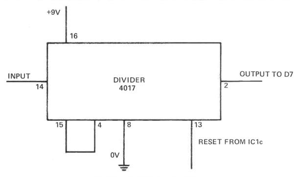
Fig 3 Alternative divide-by-two using 4017
