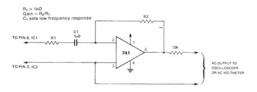
Fig 6 AC amplifier for oscillating fields
