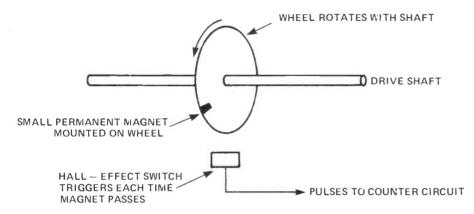
Fig 8 Simple revolution counter
