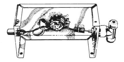
Interior view. Sampling is done via the T connector. Connection is straightforward and uses normally available components
