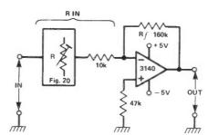
Fig 24 Digital control of gain, using the Fig 20 circuit. Gain can be varied from unity to x16, in sixteen steps
