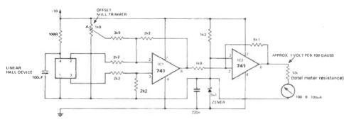
Fig 5 Simple DC amplifier for use with the 634552 device
