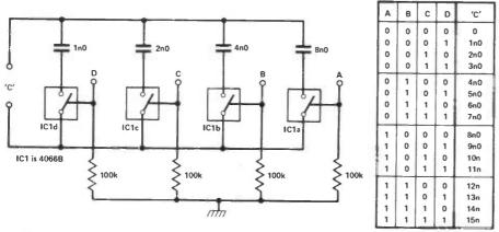
Fig 21 16-step digital control of capacitance. 'C' can be varied from zero to 15n in 1n0 steps
