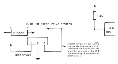
Fig 3 Using the 3020's open-collector output to drive a 6800 microprocessor's IRQ line
