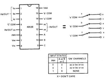
Fig 10 The 4053B triple 2-channel multiplexer/demultiplexer acts as three independent single-pole 2-way switches
