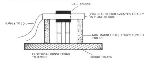
Fig 7 Location of coil and sensor
