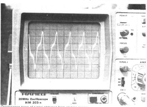
Oscilloscope trace of signal obtained from placing sensor in magnetic field of small transformer
