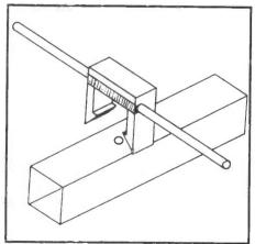
Fig 2 Fitting the element in plastic clip and mounting the clip on the boom
