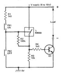
Fig 19 Alternative version of the latching power switch
