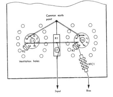
Fig 3 RF connections to valve sockets
