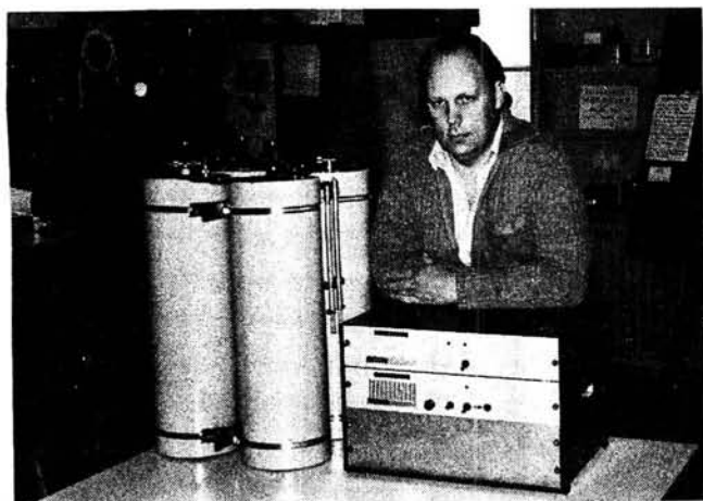
Jim GM3ZMA in the Lerwick Radio Club with the Wacom duplexer and the TX/RX/Logic unit—in fact the complete repeater except the antenna!
