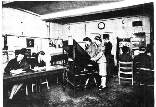
Fig. 2.5: A typical CHL receiver room. Receiver with displays in right hand corner. Plotting table centre and plotting and recording personnel on the left. CRT displays were p.p.i. (plan position indicator) and "A" trace type
