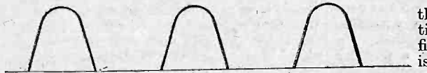
Fig. 2.—The resultant current through the rectifier as a result of applying the voltage of Fig. 1.
