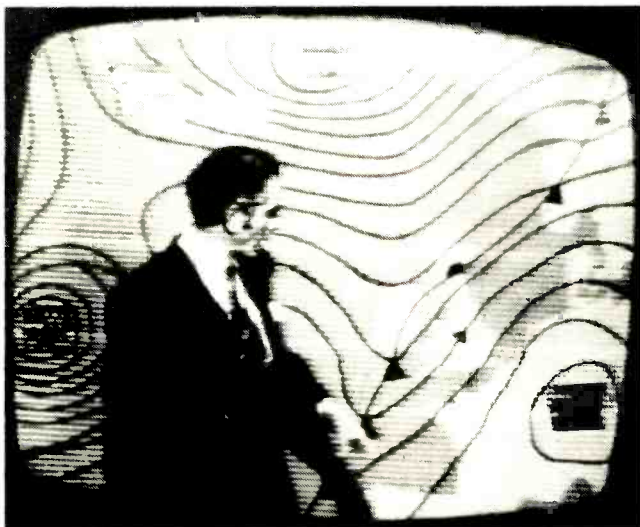
Broadcast weather chart showing an intense area of high pressure and an associated occluded front. The photograph, taken in 1974, also shows the line-pairing effect produced by interference.
