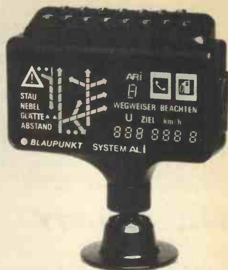
Practical application of "ALI" driver guidance system, currently tested in the Ruhr area of West Germany. The display panel supplies the following information: distance to nearest petrol station; distance to nearest telephone; road hazard warnings and route directions
