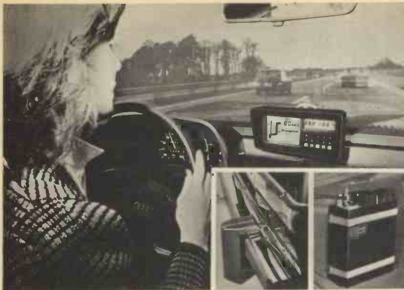
Practical application of "ALI" driver guidance system, currently tested in the Ruhr area of West Germany. The display panel supplies the following information: distance to nearest petrol station; distance to nearest telephone; road hazard warnings and route directions
