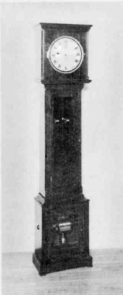
Electric clock of the type patented by Bain in 1845 (Photo courtesy Science Museum)
