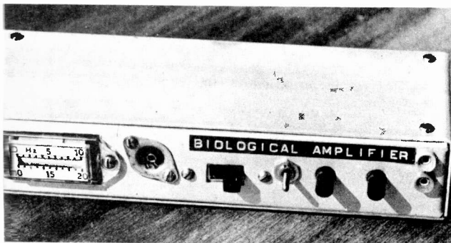
Brain rhythm frequency meter. The coaxial socket provides a connection to the visual feedback unit
