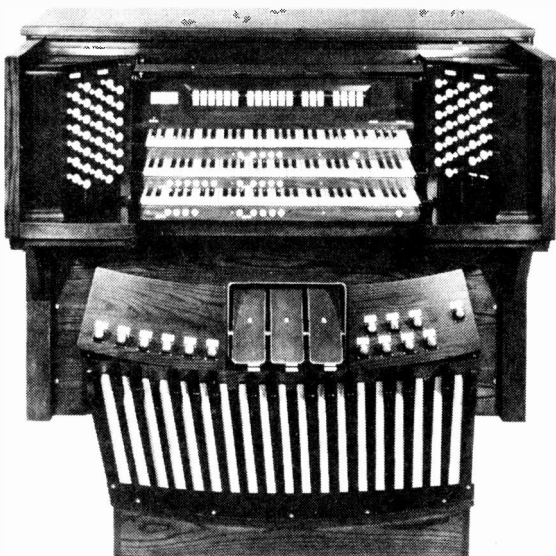
Fig. 1. The three manual Conn Custom organ has independently tuned oscillators for each note. These can provide at least three different waveforms for tonal synthesis of a church or concert pipe organ.
