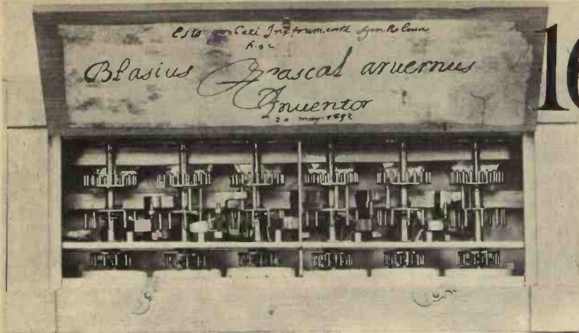
Replica of Pascal's Calculating Machine . (Crown Copyright. Science Museum, London)
