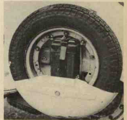
Spare wheel and battery compartment on the Sportique model
