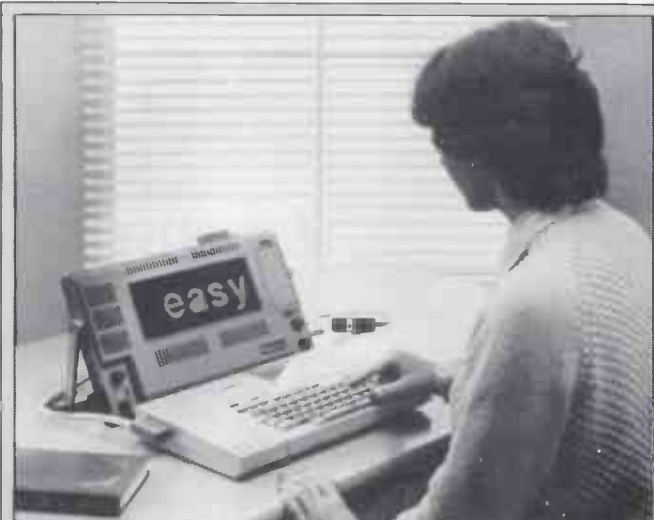
The reason the word 'easy' is displayed in two-inch high letters is that the operator is partly blind. The ViewScan system uses the Epson micro and a little camera to expand the word from paper, or from the computer.
