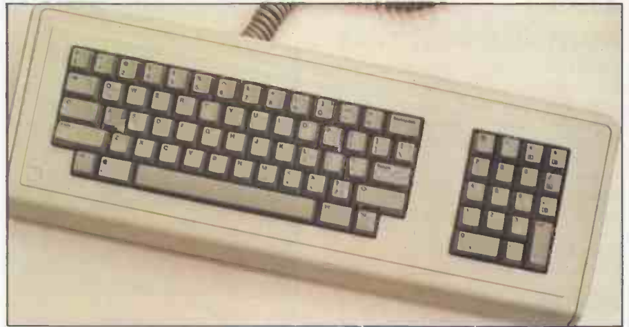
All 76 keys are programmable but the mouse is used to issue most commands.
