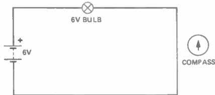
Figure 2. When the circuit is completed the needle of the compass will jump to a new position. As the circuit is disconnected the compass needle will once again point north.
