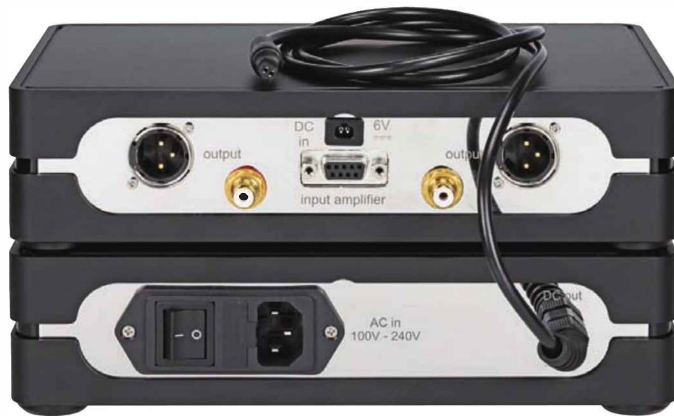
Absolute Phono 'outside' and below its power supply. Inputs lie at centre: d.c. power and a multi-pin socket for arm connection.
