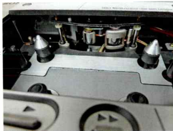
Two pinch-rollers (with conic 'caps') wrap the tape around the EL-7's three heads during record/play-back
