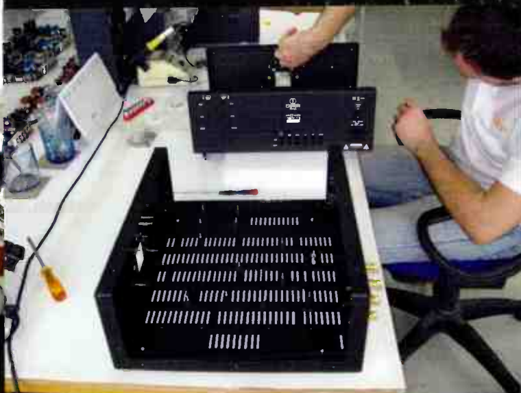
▲ All of Canor's products are hand assembled. These are the cases for the TP 134 amplifier having their sockets fitted.
