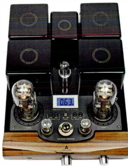
A blue display screen shows bias voltage, for easy bias adjustment.
