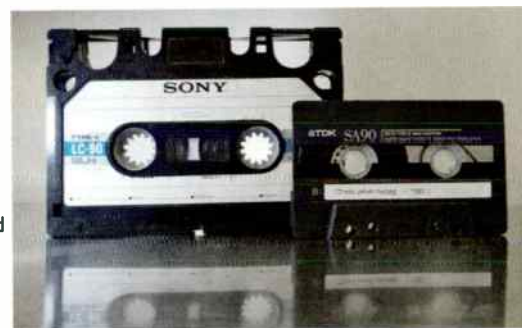
As we see here, the Elcaset is considerably larger than a normal Philips cassette
