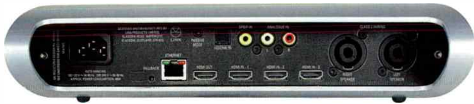
HDMI sockets pass through video, whilst playing audio.
