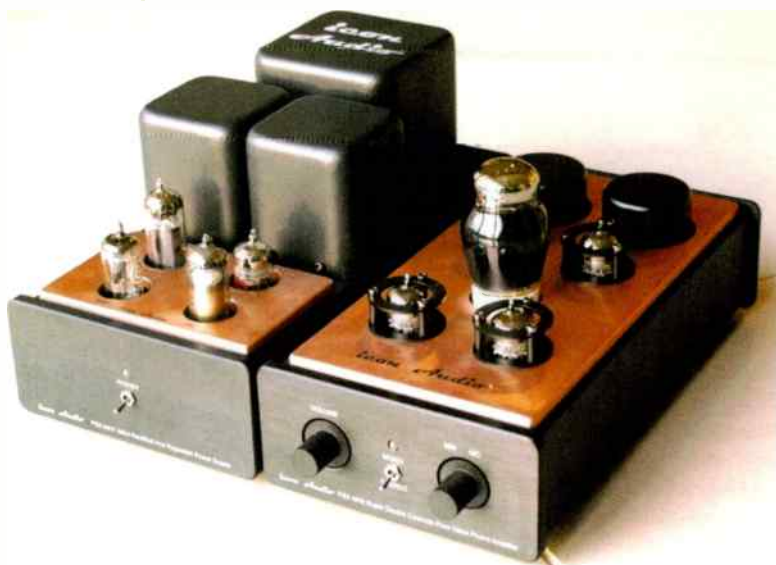
Early production photos. Showing PS3 upgraded version with JJ and Treasure valves, and Jensen Copper foil in paper and oil caps, Icon Audio W transformers
