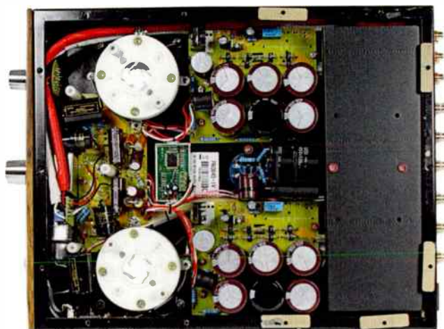
Giant 845 ceramic valve bases dominate the underside.
