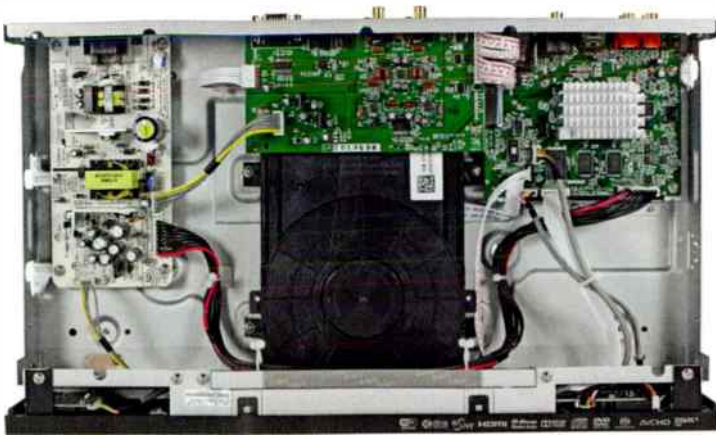
Switch-mode power supply at left, disc tray centre and comprehensive signal processing, needing a heatsink, at right.
