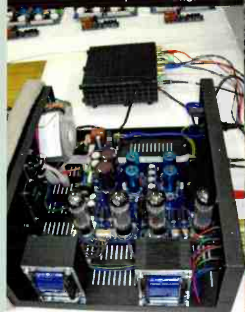
▼ A completed TP134 amplifier connected up for testing.
