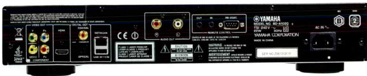
The rear carries stereo audio outputs, Component and Composite video outputs HDMI and a network connection, plus S/PDIF digital audio.
