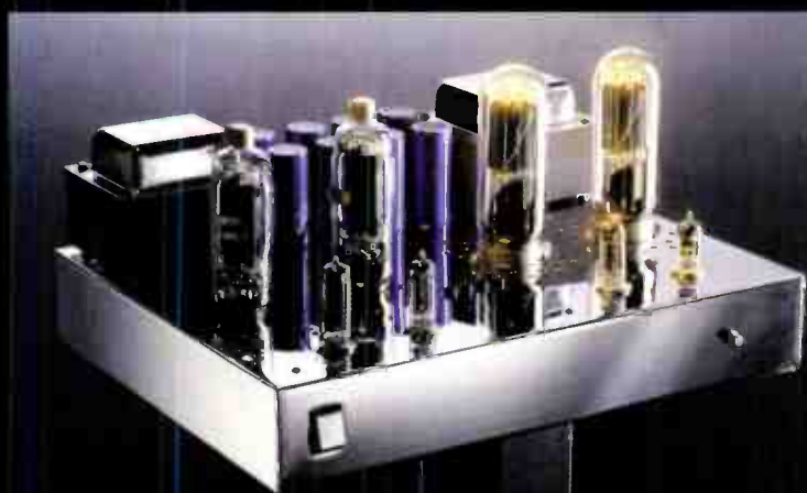
A World Audio Design 211 amplifier, using 1919 transmitter valves: the VT211. Take cover.
