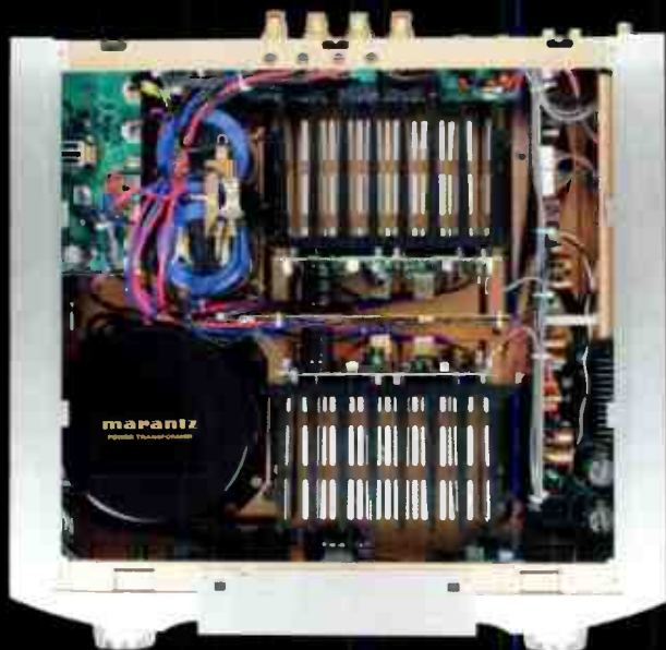
Copper plating a steel chassis eliminates eddy current induced hysteresis distortion. It's a popular technique in Japan, on upmarket models like the PM11 seen here.
