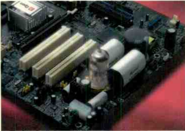
Something you thought you'd never see- the PC that glows in the dark! The single Sovtek 6922 in its full glory...
