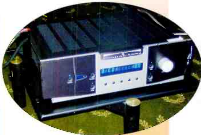
Balanced Audio Technology, an American company, specialise in complex valve amplifiers. Here they were showing a new MOSFET/tube hybrid, the VK300x.
