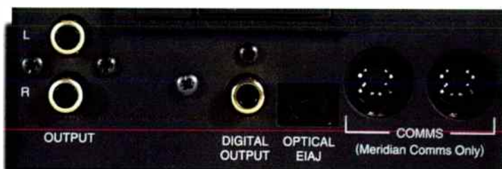
Tidy rear panel offers a host of analogue and digital audio outputs plus a COMMS link to connect to other Meridian electronics
