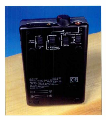
Controls on the TCD-D100's rear include Short and Long Play modes as well as 44.1/48kHz sampling rates. Other options relate to microphone and line inputs.
