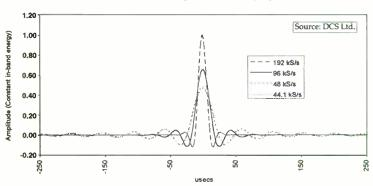
Figure 2 - Energy spread for different sampling rates
