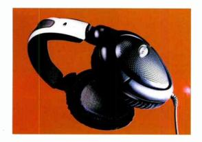
Duofol. This is a laminate of two Mylar films which yields a light, rigid diaphragm aimed at providing a controlled sound even at high volumes. Lightweight alloy wire on the voice coil is matched by neodymium/iron magnets, with three metres of Kevlar-reinforced OFC lead (topped off by a 3.5mm stereo minijack and a 0.25in. adaptor) providing the finishing touch.
