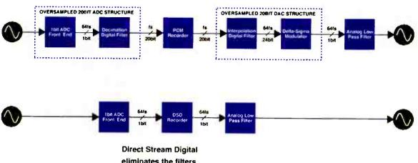
eliminates the filters and records the original 1-bit signal directly.
