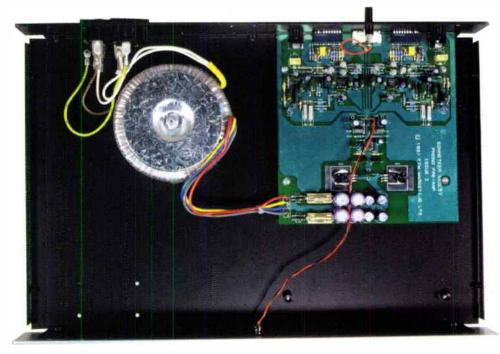
The Sedley's casework is sparsely populated. On the small PCB with its short signal paths are the staggered reservoir caps, active ground circuitry and discrete input stage.
